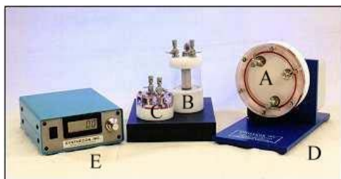
Figure 2.2 The rotary cell culture system
