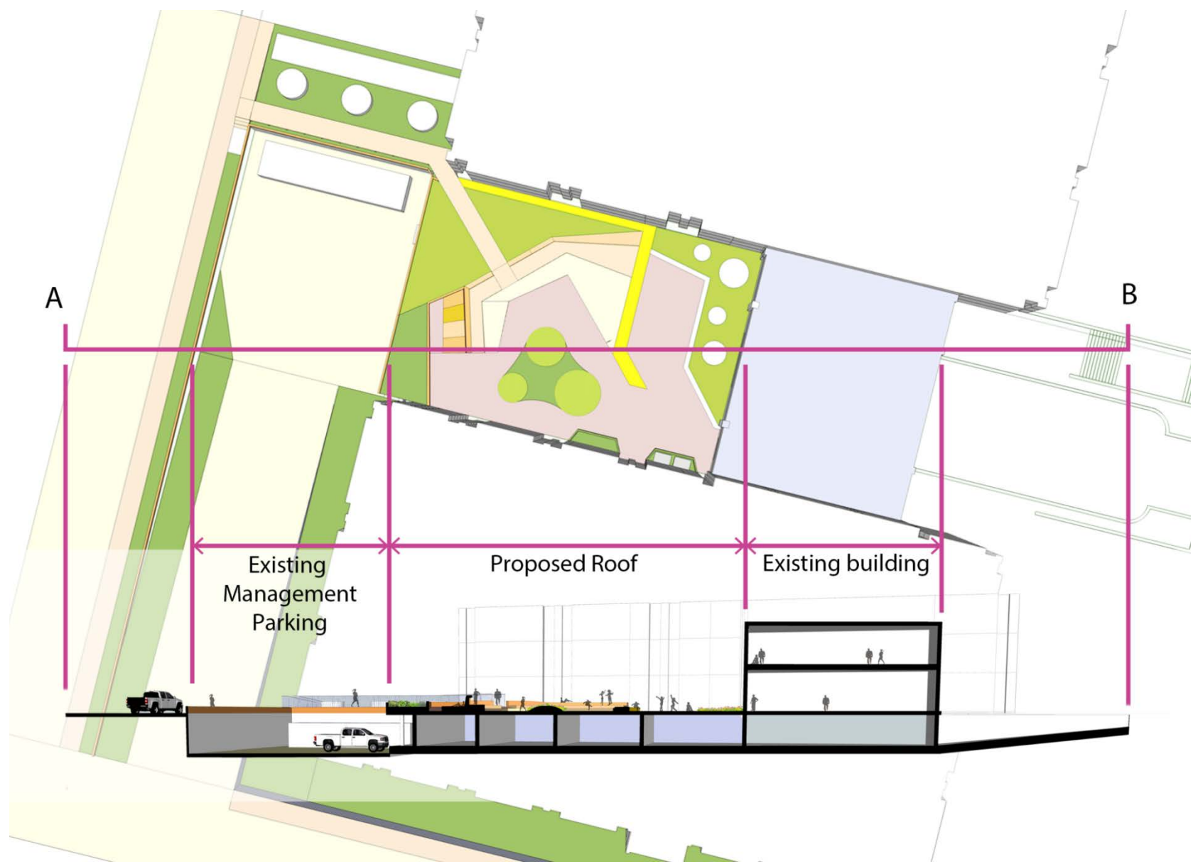
Figure 5.11 Boyd green roof section A-B
