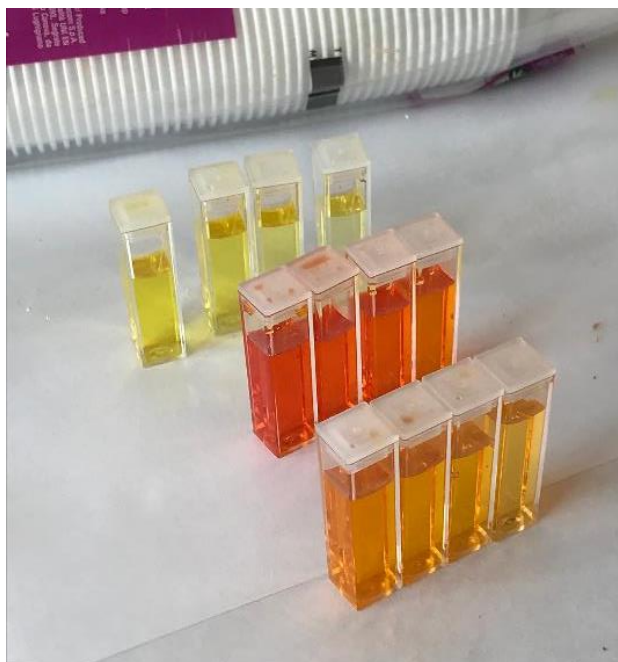
Figure 6.17. Serial dilutions prepared by Chemistry in the Arts students using the azo dyes in Cortona, Italy. From top to bottom: phenol dye, ethyl orange, and methyl orange. The cuvettes are arranged in order of most concentrated (left) to least concentrated (right) in each row.
