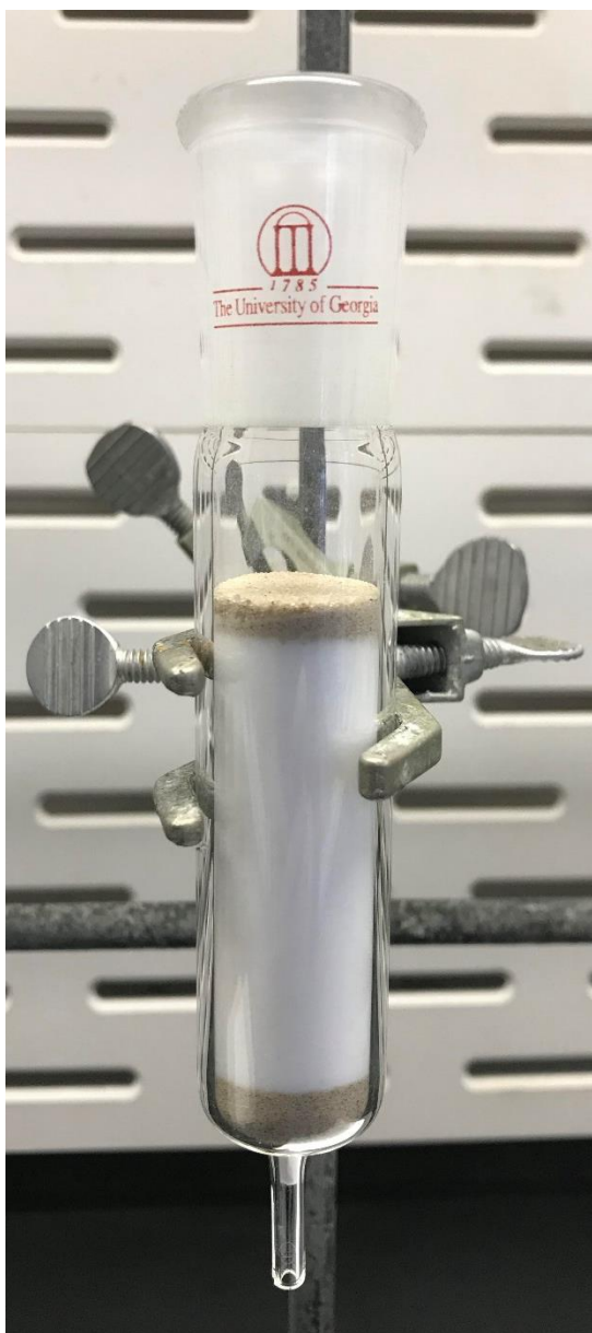
SI Figure 4.2. Example column prepared by students in Spring 2018. The columns were made by the Scientific Glassblowing Shop at the University of Georgia using 24/40 tubing. The column pictured is approximately 6.5 inches long.
