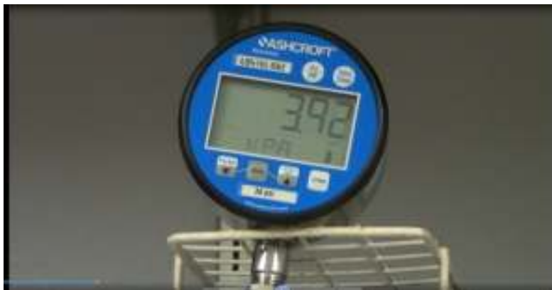
Figure 2.9: Pressure gauge set up for pressure test of DIM. Note units set for kPa.
