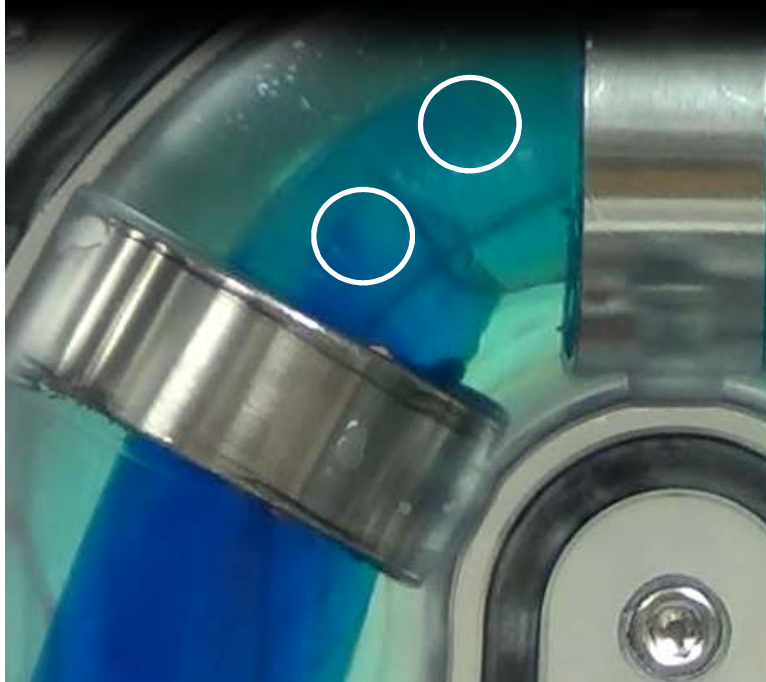
Figure 3.12: Close up of DIM right after a contraction. Note two faint vortices formed right after the contraction, which went away less than a second after contraction.
