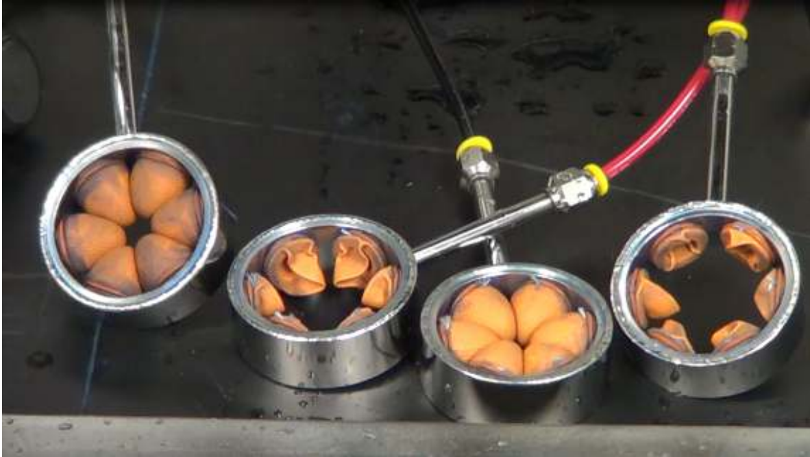
Figure 2.7: Close-up of segmentation mechanism in DIM. These rings can contract to a diameter of roughly 1 cm. Inner diameter of contraction rings is 3.5 cm.
