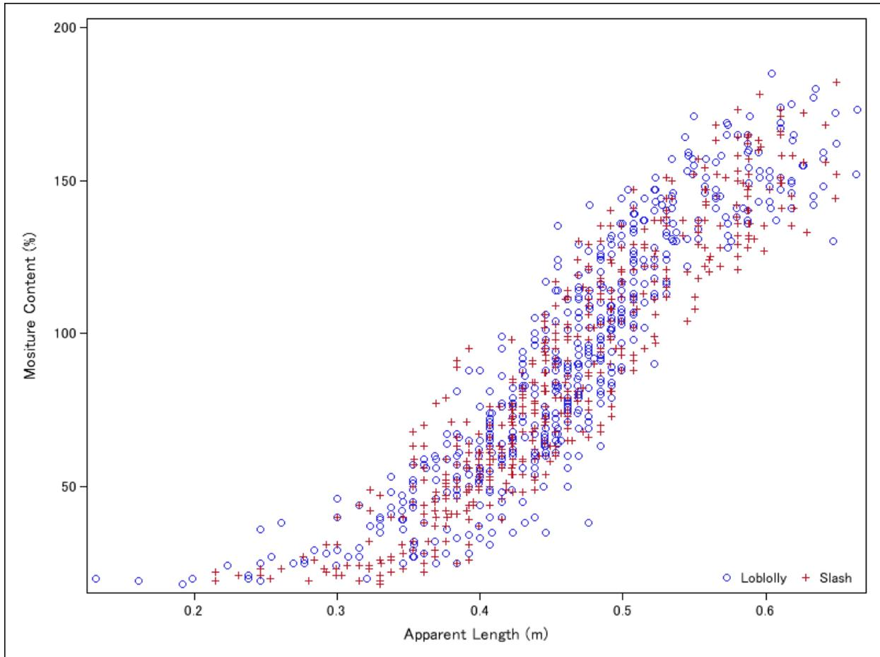
Figure 2.1. Relationship between MC and apparent length for *P. elliottii* (slash pine) and *P. taeda* (loblolly pine) from the Lower Coastal Plain. Measurements were collected with the TV220 TDR.
