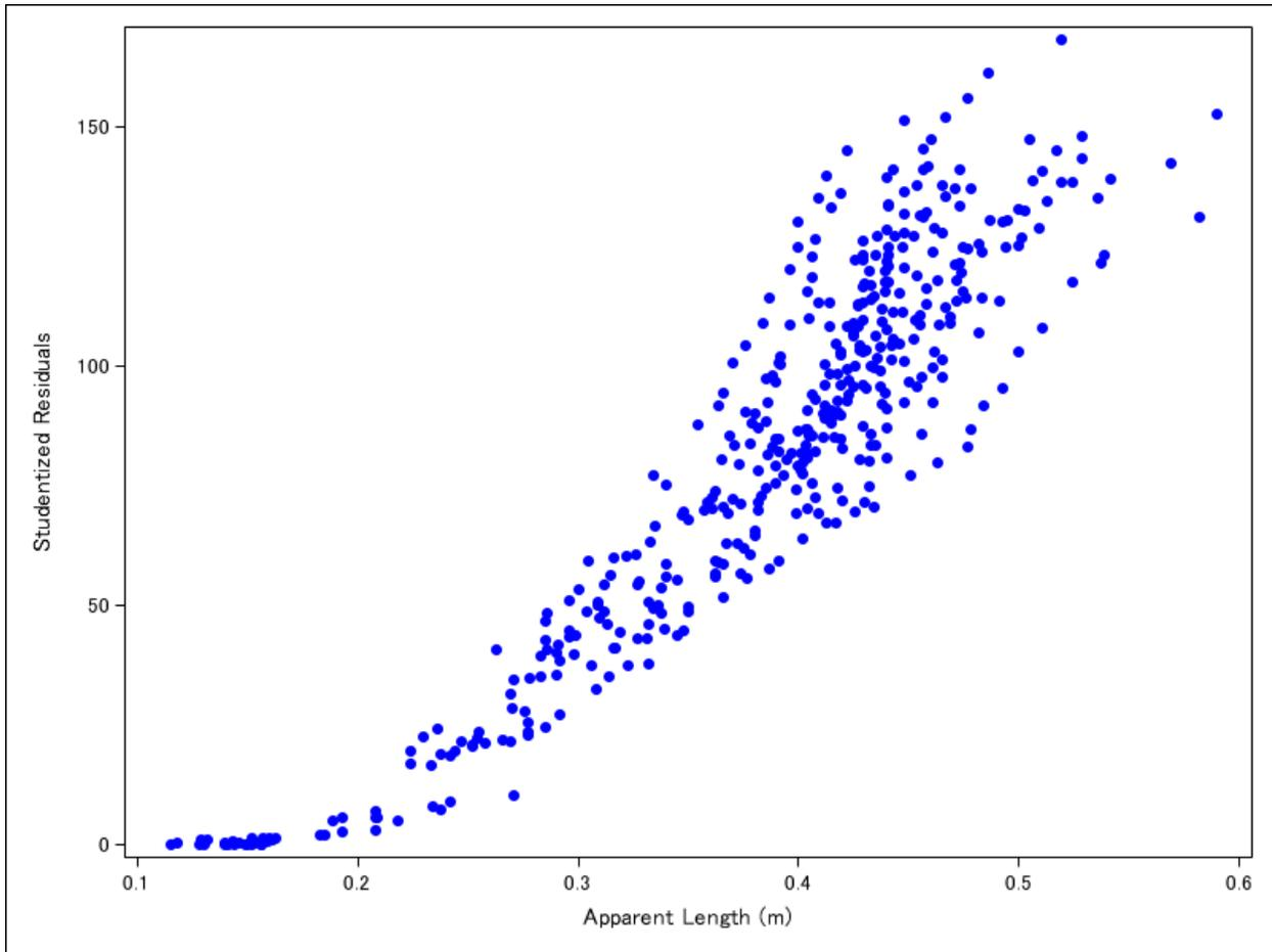
Figure 2.5. Relationship between MC and apparent length for *P. taeda* (loblolly pine) from the Piedmont. Measurements were collected with the Tektronix 1502C cable tester.
