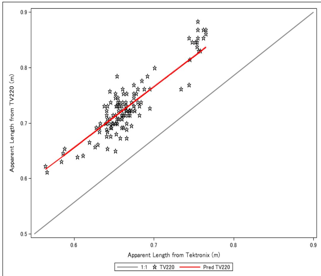
Figure 2.8. Reference length (m) for probes constructed for this research measured with the Tektronix 1502C and adjusted to the Cable Scout TV220 (the regression line for the conversion is shown).
