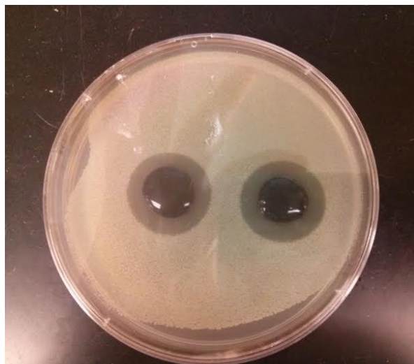
Figure 5.6. Incubation of a 6 wt% pDMA hydrogel with S. aureus . The gel showed a zone of inhibition when loaded with 5.1 \text{ mg} \cdot \text{mL}^{-1} potentiated neomycin sulfate.
