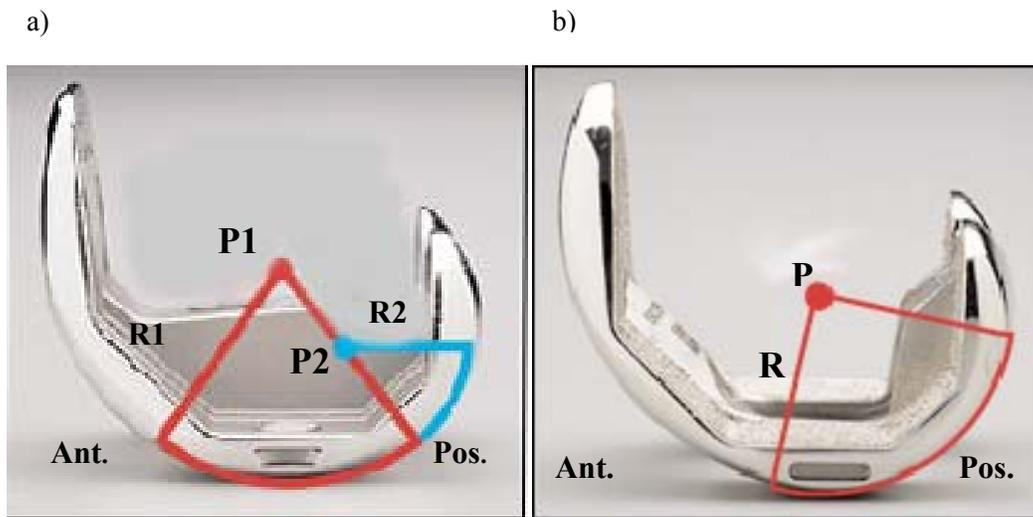
Figure 3.1. Lateral views of left knee femoral components of the a) M-RAD TKA and b) S-RAD TKA. P1, P2, and P represent the centers of flexion/extension rotation, and R1, R2, and R represent the corresponding radii of rotation. (Courtesy of Stryker-Howmedica-Osteonics Inc.)
