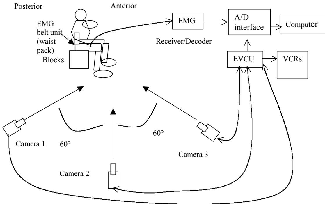
Figure 4.2. Experimental setup for the stand-to-sit task.
