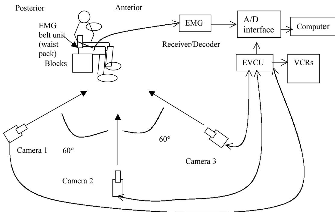
Figure 3.2. Experimental setup for the sit-to-stand task.
