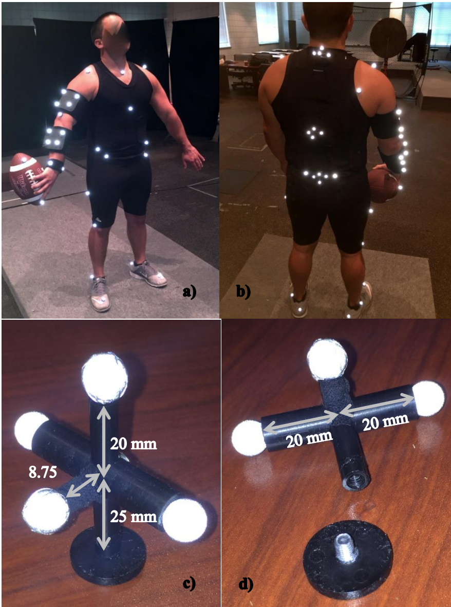
Figure 5.2 — Marker set. (a) Front view (b) and back view of the full marker set used for motion capture. (c) An assembled example spinal marker cluster set. (d) An unscrewed spinal marker cluster set. Marker sets placed on the C7, L3, and T8 vertebrae, were made of four 9.5 mm-diameter markers attached to a base consisting of a 6.6 mm-diameter vertical plastic rod crossed with a 9.7 mm-diameter horizontal plastic rod; a 3 mm-diameter screw, protruding from the 3 marker plane, covered with black tape; and a 19.1 mm-diameter solid plastic base with a 4 mm-diameter screw projecting from it into the horizontal rod. The base was placed on the skin and fed through a small hole in the garment.
