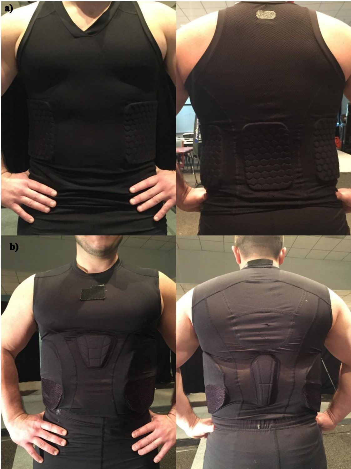
Figure 4.1 — The rib protectors tested in this study: (a) soft-rib and (b) hard-rib. All logos were covered to avoid bias due to brand. Padding on the sternum and along the spine was made of a harm foam, not plastic like the rib inserts. The control condition consisted of the hard-rib compression shirt without the plastic inserts.
