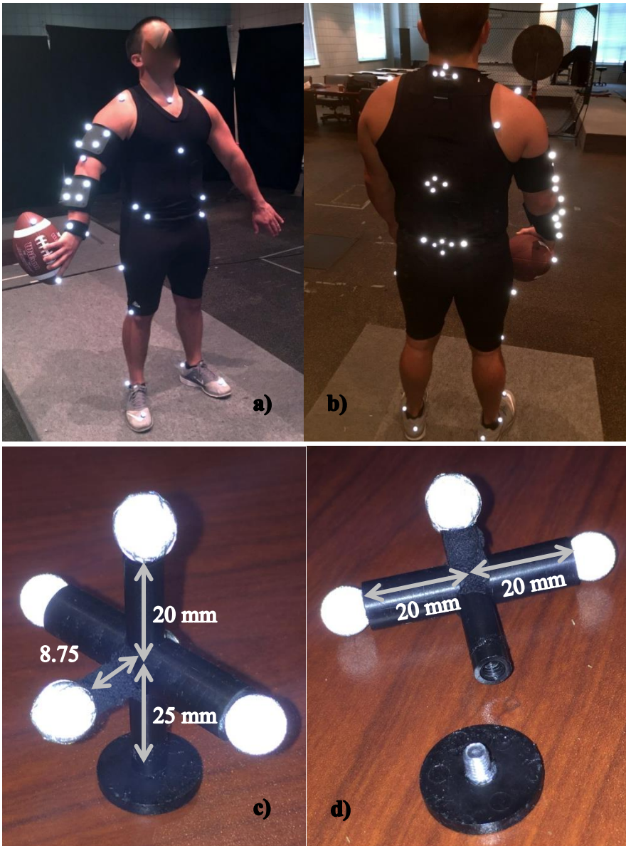
Figure 4.3 — Marker set. (a) Front view and (b) back view of the full marker set used for motion capture. Additional markers not used in this study were placed on the participant. (c) An assembled example spinal marker cluster set. (d) An unscrewed spinal marker cluster set. Marker sets placed on the C7, L3, and T8 vertebrae, were made of four 9.5 mm-diameter markers attached to a base consisting of a 6.6 mm-diameter vertical plastic rod crossed with a 9.7 mm-diameter horizontal plastic rod; a 3 mm-diameter screw, protruding from the 3 marker plane, covered with black tape; and a 19.1 mm-diameter solid plastic base with a 4 mm-diameter screw projecting from it into the horizontal rod. The base was placed on the skin and fed through a small hole in the garment.
