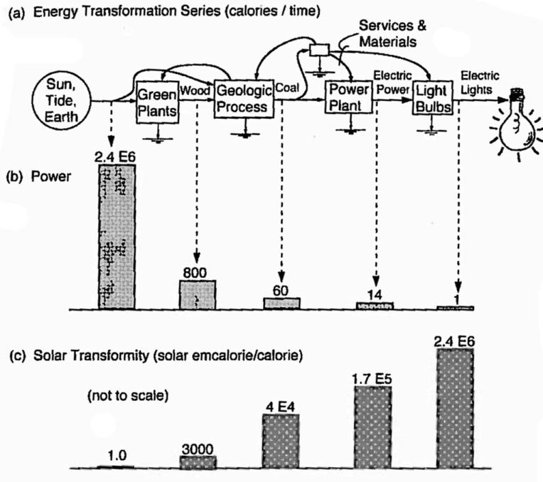
Figure 2.4. Energy Transformation (a) Energy Transformation Series from solar energy to electrical lighting; (b) Bar graph depicting power lost with each transformation; (c) Solar emcalorie required per calorie for each step in the transformation series (Odum 2007, 70).
