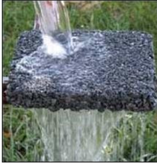
Figure 5: Pervious Pavement: Water is allowed to pass through porous pavement, thus increasing stormwater infiltration 117
