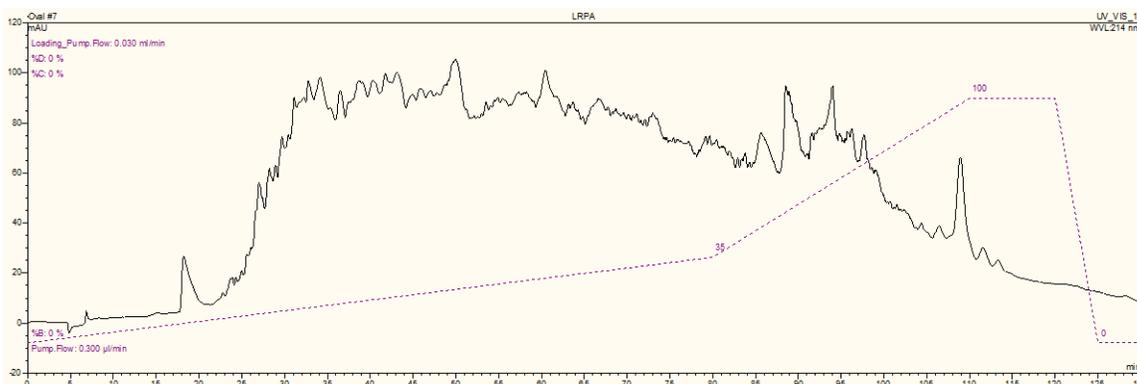
**Figure 2.1** Sample chromatogram showing the elution gradient used. The x-axis is time (min) and the y-axis is the measured absorbance in arbitrary units. The sample shown here is the mixture of peptides from a proteome sample derived from a whole cell lysate from *Methanococcus maripaludis*  $\Delta\text{lrp}$ .
