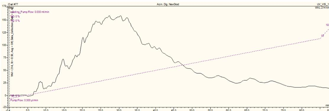
**Figure 3.2** HPLC Separation of the proteome digest of *Acinetobacter baylyi* ADP1. The mobile phase B gradient is shown as a dotted line.
