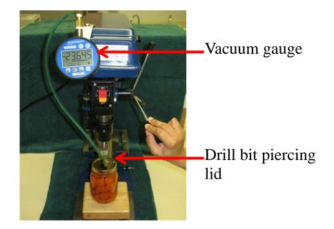
Figure 3.4. Vacuum gauge in use on drill press for measuring headspace vacuum in jars canned with metal and plastic lid systems
