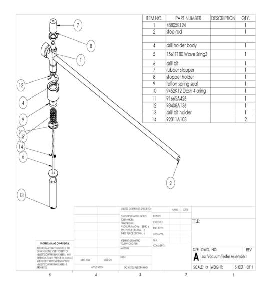
Figure E.1. Parts of the vacuum gauge
