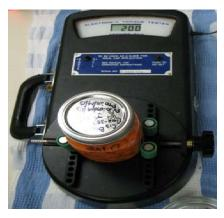
g. Screw band tightened using Torque tester
