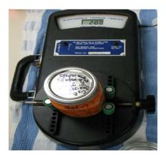
g. Screw band tightened using Torque tester
