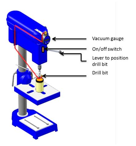
Figure. 3.3. Vacuum gauge mount on 5-speed drill press for measuring headspace vacuum with home canning metal and plastic lid systems
