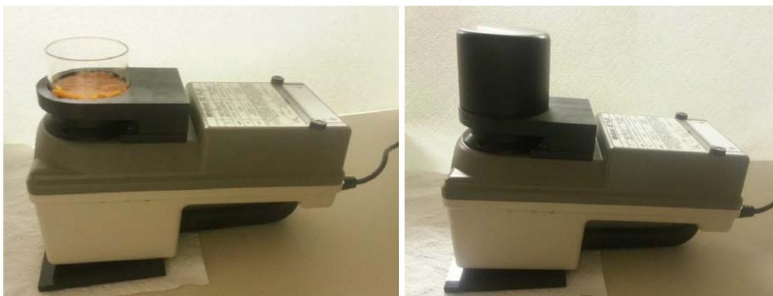
**Figure. 3.5. Measuring color of the food using the HunterLab Colorimeter**
