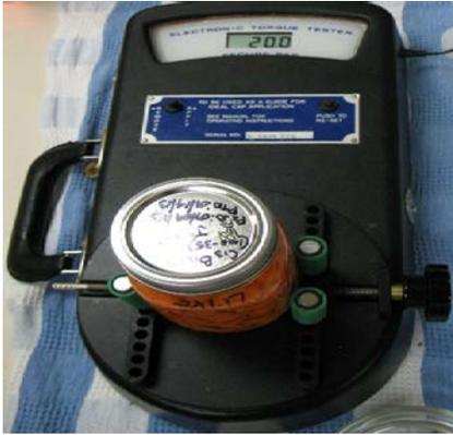
**g. Screw band tightened using Torque tester**
