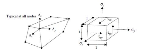
Figure 4—Volume Element [Fu et al., 2015]
