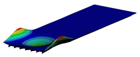
Figure 23—Mode 11 Total Deformation
