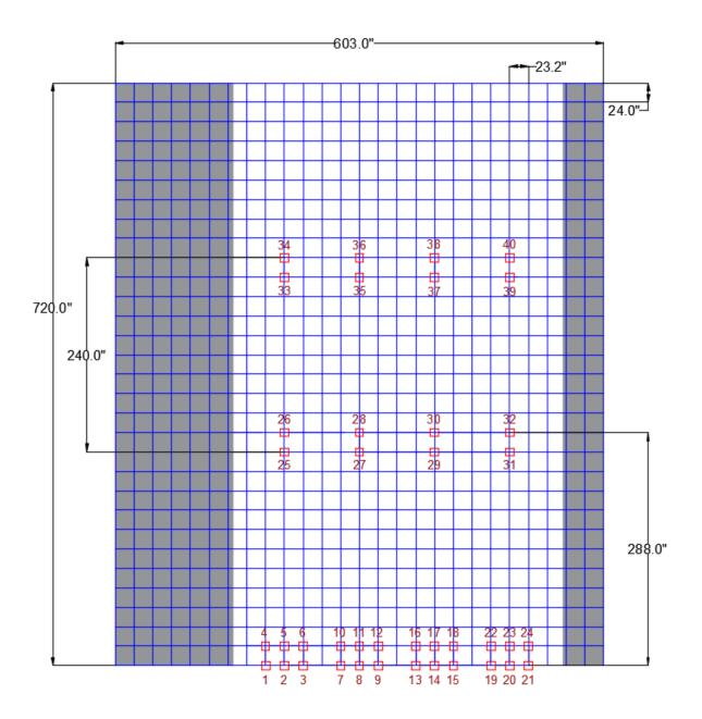
Figure 26—Unit Load Layout
