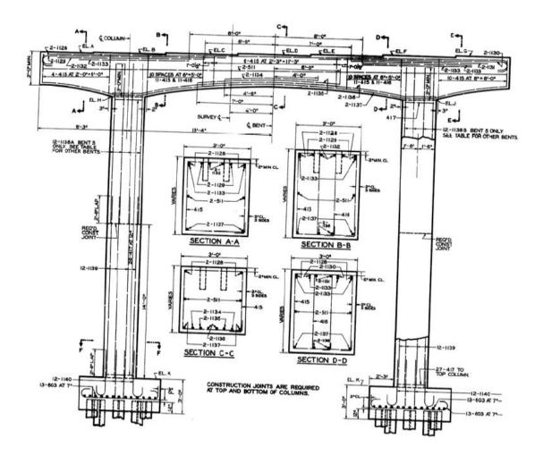
Figure 13—Bent Elevation View Detail
