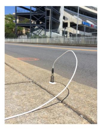
Figure 24—Accelerometer Setup
