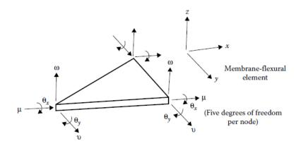
Figure 3—Plane Shell Element [Fu et al., 2015]
