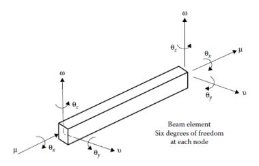
Figure 2—Beam Element [Fu et al., 2015]
