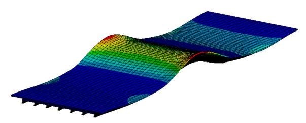
Figure 22—Mode 4 Total Deformation
