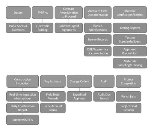
Figure 7—Paperless Processes Created by e-Construction [Pavement Interactive, 2016]
