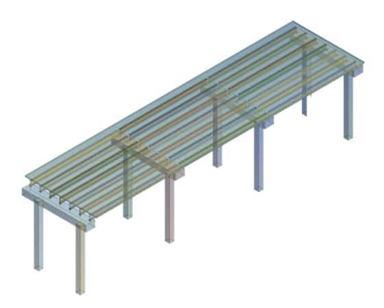
Figure 18—Isometric View of Bridge Model
