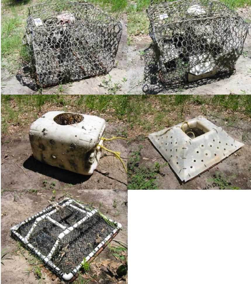
Figure 2.2. Standard crab trap (top left), Modified crab trap (top right), Alcohol container trap (middle left), Plastic pyramid trap (middle right), Mesh pyramid trap (bottom left).
