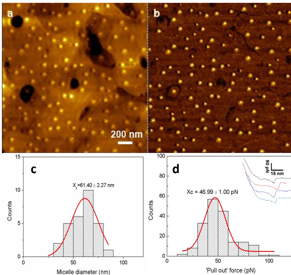
**Figure 2.8:** AFM measurements on micelles adhered on a gold surface: a) topography image, b) phase image, c) the distribution of the micelle diameter and most probable value from Gaussian fitting, d) force histogram and most probable ‘pull out’ force, the typical force distance curves were exemplified in the inset.
