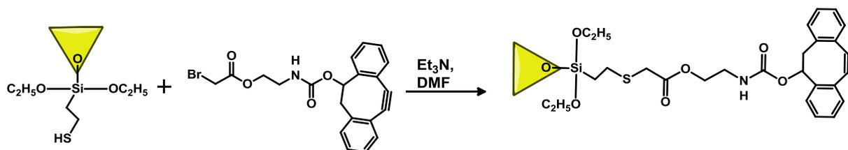
**Scheme 2.5:** Modification of AFM Tip with DIBO moiety
