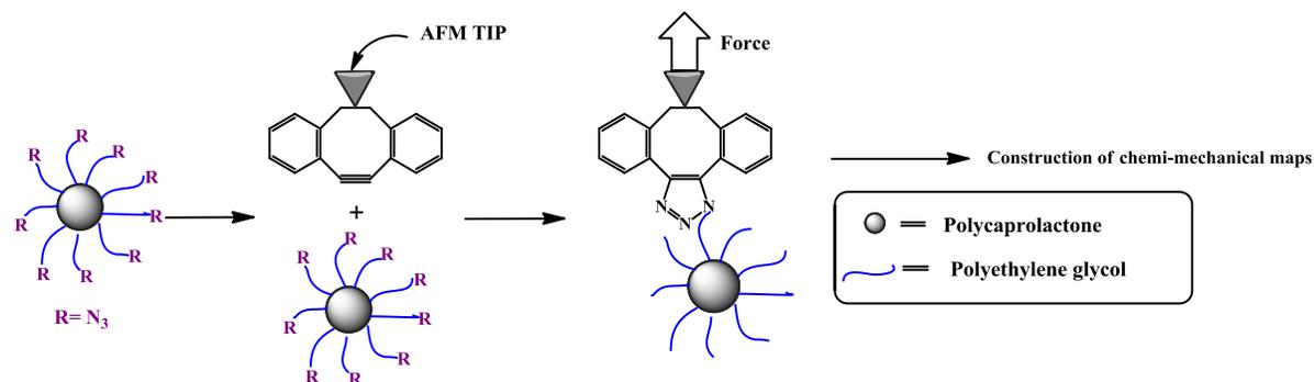
**Scheme 2.6:** Schematic illustration of the DIBO modified tip and its use in AFM studies
