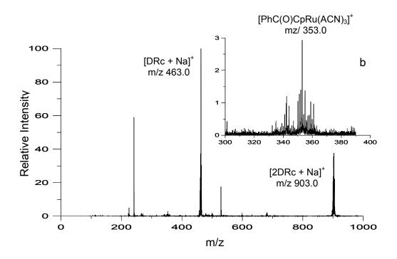
Figure 3.25: Mass Spectrum of Benzoylruthenocene in CCI<sub>4</sub>
