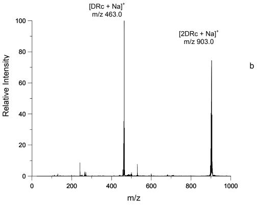
Figure 3.23: Mass spectra of Benzoylruthenocene in ACN
