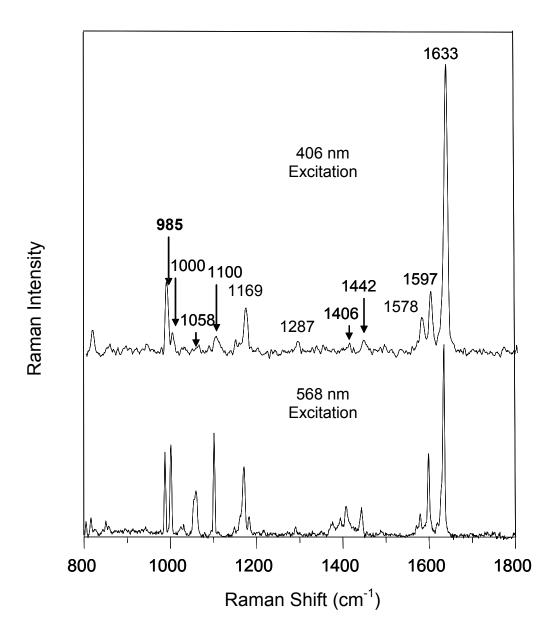
Figure 3.16: Raman Spectra of 1,1'-Dibenzoylruthenocene
