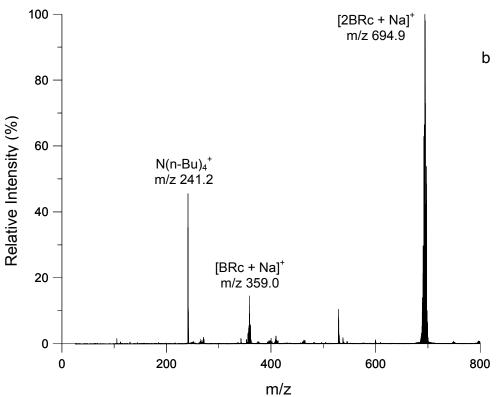
Figure 3.24: Mass Spectra of 1,1'-Dibenzoylruthenocene in CCI<sub>4</sub>
