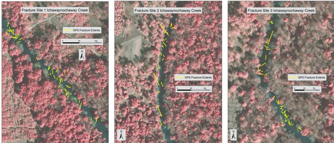
Figure 4.7. Remote sensing view of location, direction and extent of stream bedrock fractures (joints) measured within Ichawaynochaway Creek (n=125) in the Lower Flint River Basin, southwestern Georgia, USA, projected on 2011 National Agriculture Imagery Program (NAIP) aerial near infrared photography in ArcGISv.9 (downstream to upstream: Fracture site 1,2, and 3).
