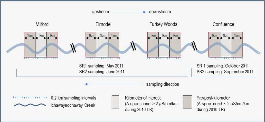
Figure 3.2. Experimental study design for fine scale sampling of short runs (2011 SRs) on Ichawaynochaway Creek at 200 meter (0.2 km) intervals.
