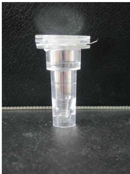
Figure 3- 2. Setup for Second Heat Escape Extraction Method. This heat escape extraction setup contained two plexiglass rings on top of wire mesh and an additional plexiglass ring on top of a tube.
