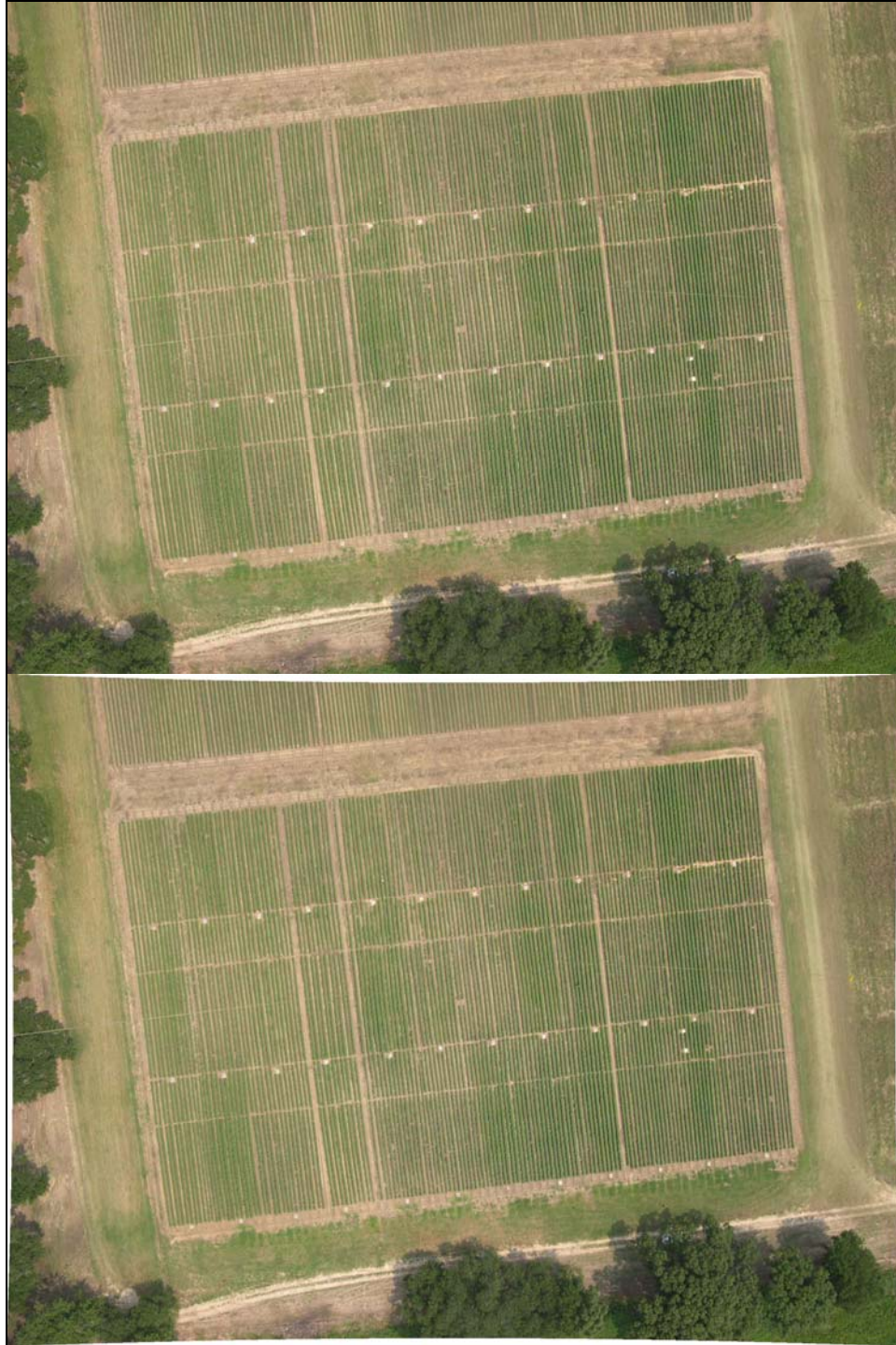
Fig. A.2. Image before (top) and after (bottom) image correction. Image correction was performed using the lens correction filter in Adobe Photoshop with a 3.5% correction filter. The black border around the images emphasizes the correction required to minimize the barrel distortion.
