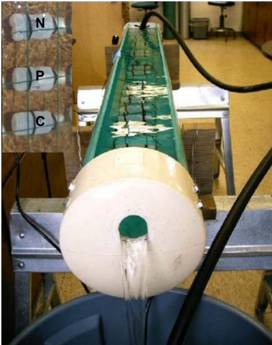
Figure 2.2. Experimental Creek. Trough cut from 20-cm diameter PVC pipe. 60-mL bottles filled with N+P solution with glass fiber filters are oriented sideways 7.5 cm apart just under the surface of the water. Water is circulated by submersible pump in the 167-L container (at the bottom of the picture) with 2.5-cm diameter hose extended to elevated end of the trough (at the top of the picture). Inset: Nutrient-diffusing bottles held under the surface of the water.
