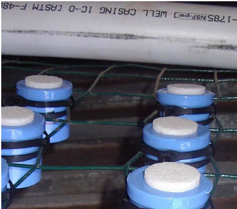
Figure 2.3. Agar vials attached to the periphytometer. The vials are oriented so the porcelain disk is parallel to the surface of the water.
