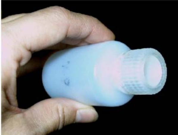
Figure 2.1. A 60-mL bottle with 1.5-cm hole cut in the lid. Dialysis membrane and glass fiber filter are held in place between the mouth of the bottle and the lid.
