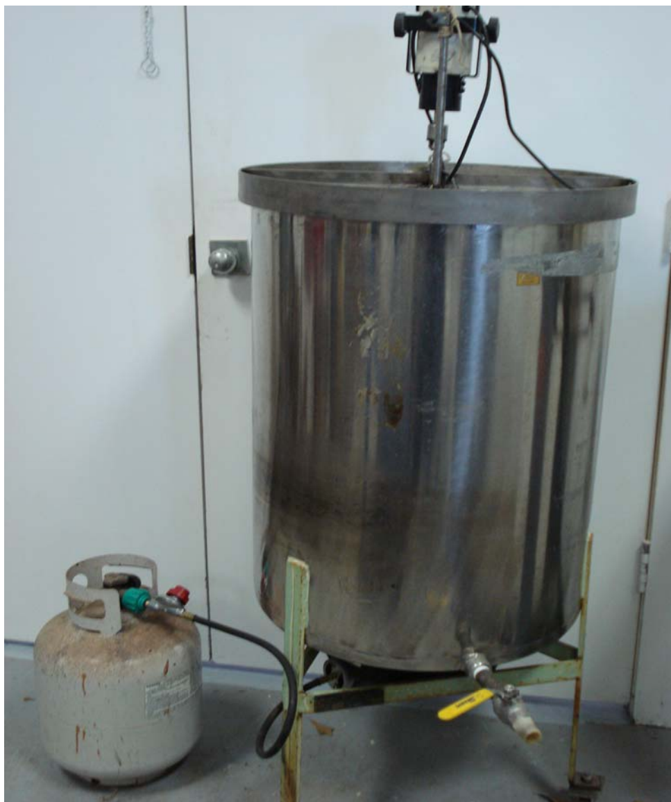
Fig 3.3 Extraction tank with gas fired heater
