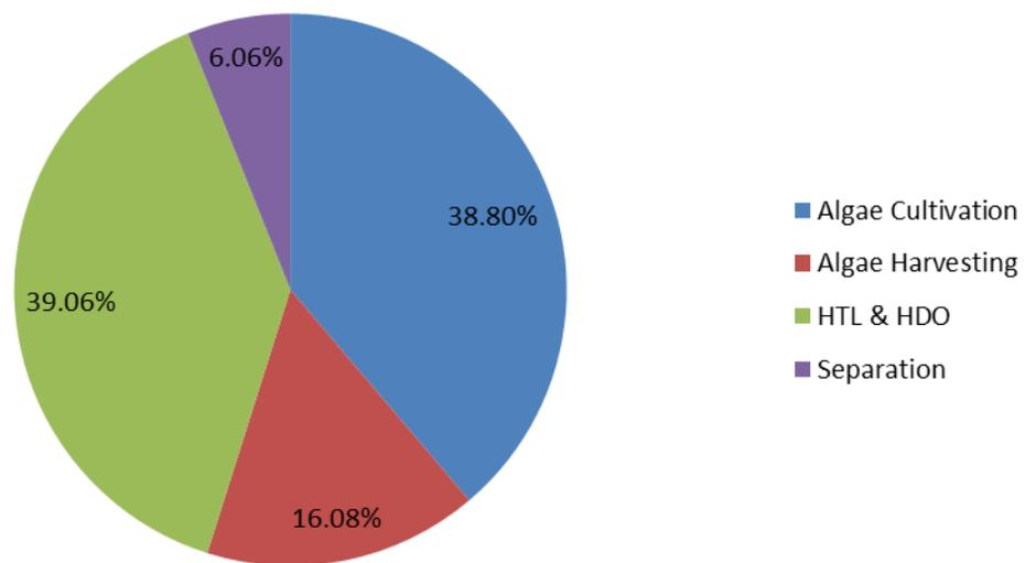
**Figure 3.4. Breakdown of the capital cost of the algal bio-crude plant**
