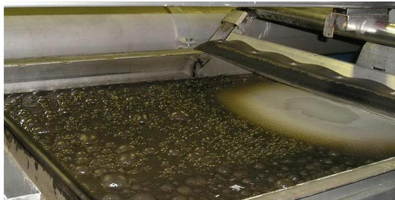
**Figure 2.2. Flotation device from BIO-AQUA, Denmark**
