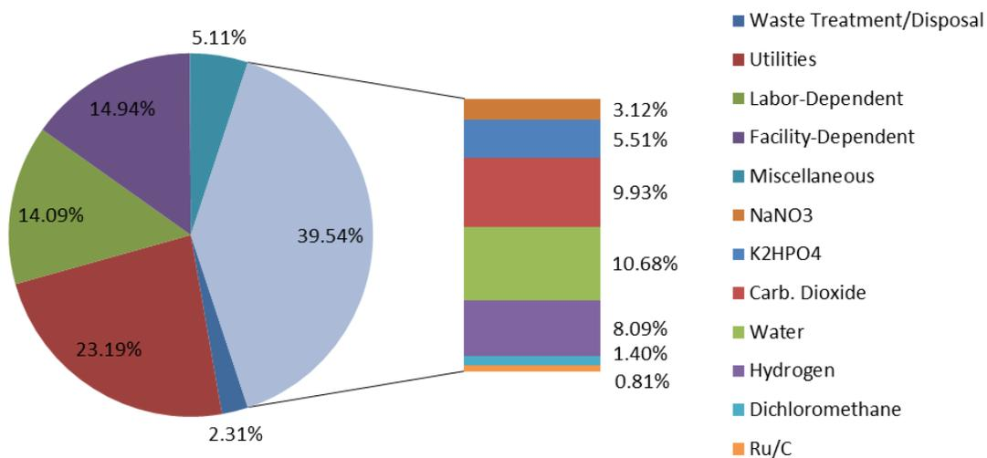
**Figure 3.5. Breakdown of the operating cost of the algal bio-crude plant**
