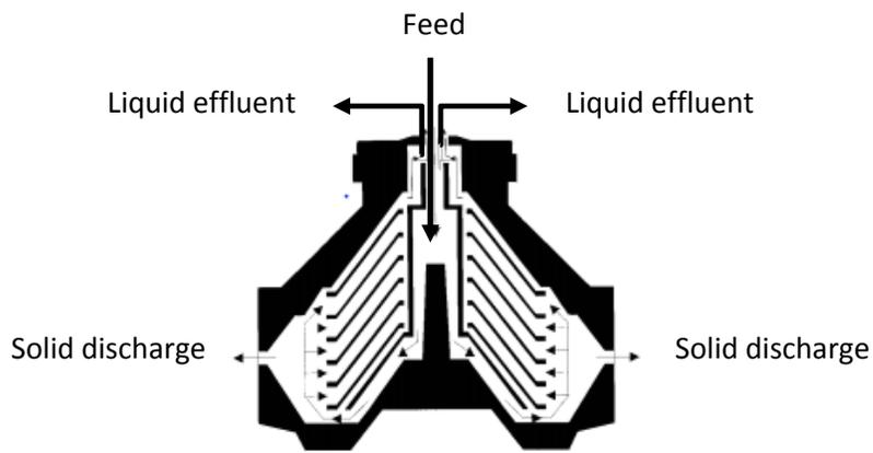
**Figure 2.4. Schematic diagram of a disc stack centrifuge (Maybury et al., 1998)**
