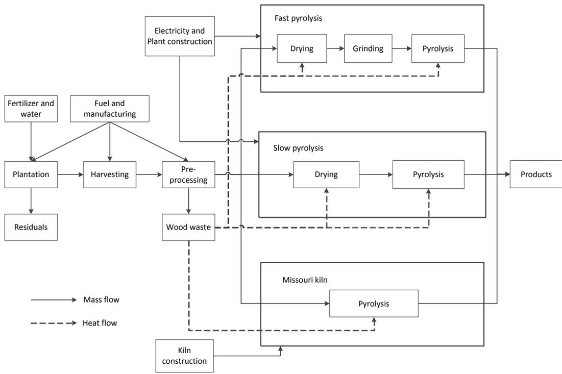
**Figure 5.1. System boundary of different scenarios to produce biochar or bio-oil from southern pine**
