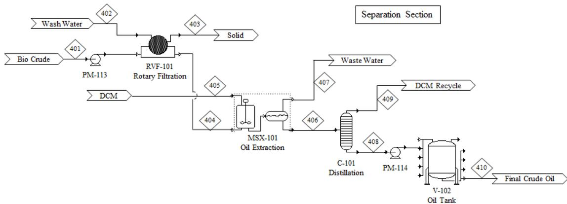
**Figure A.5. Flow diagram of the separation section**
