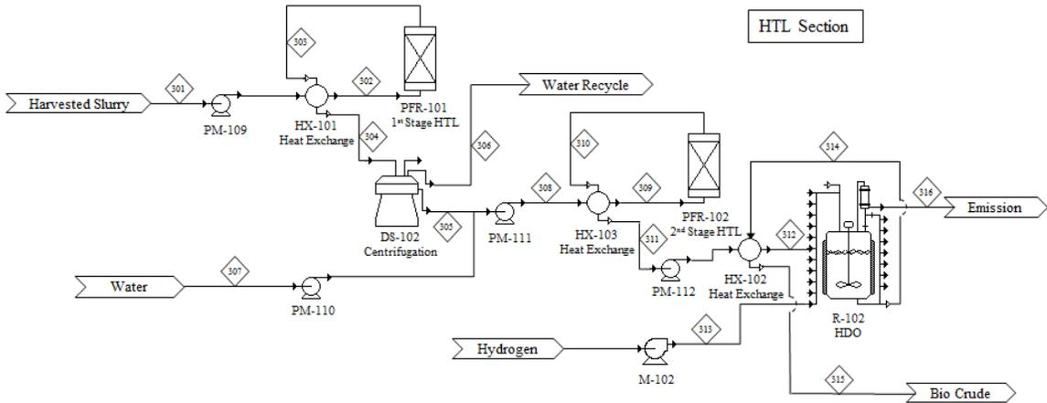
**Figure A.3. Flow diagram of the HTL & HDO section**
