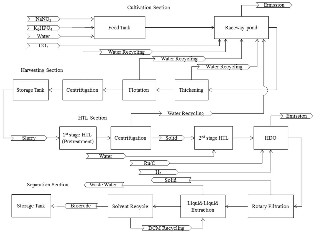
**Figure 3.1. Simplified flow diagram of the overall process**
