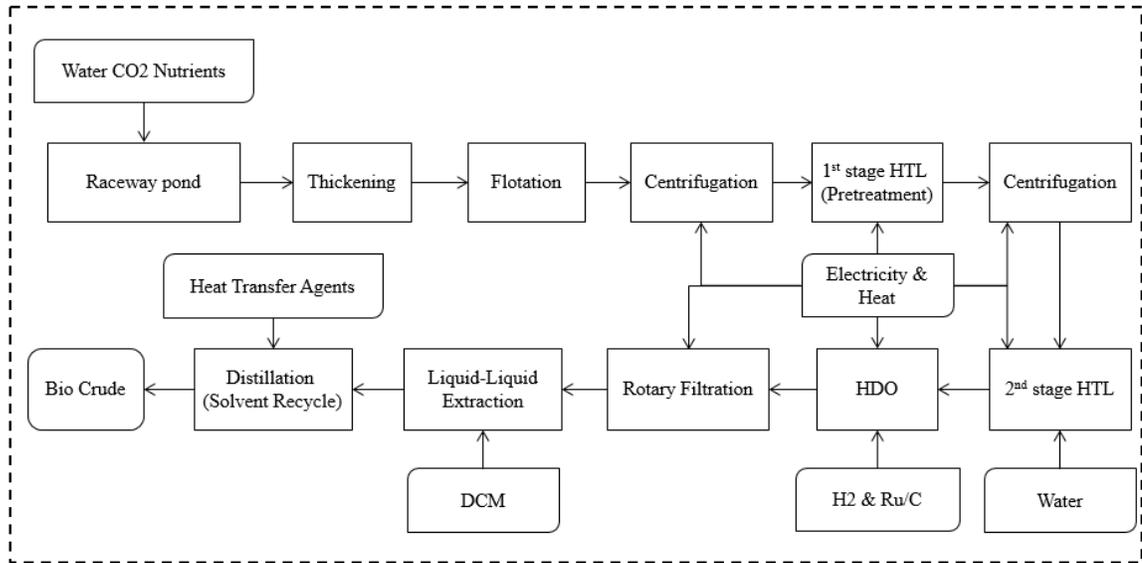
**Figure 4.1. System boundary of life cycle assessment of algae liquefaction technology**
