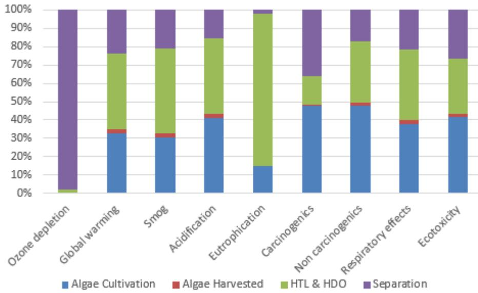
**Figure 4.2. Environmental impacts of per gallon of algae liquefaction biofuels**
