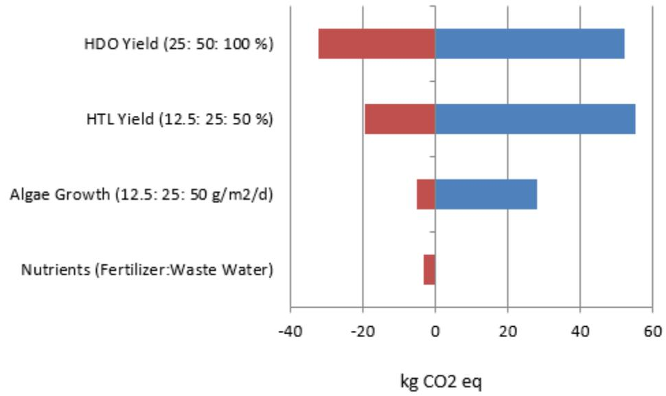
**Figure 4.4. Sensitivity analysis of global warming impact of algae liquefaction technology**
