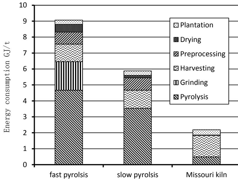
**Figure 5.2. Breakdown energy consumption for each process of biochar production from three scenarios**
