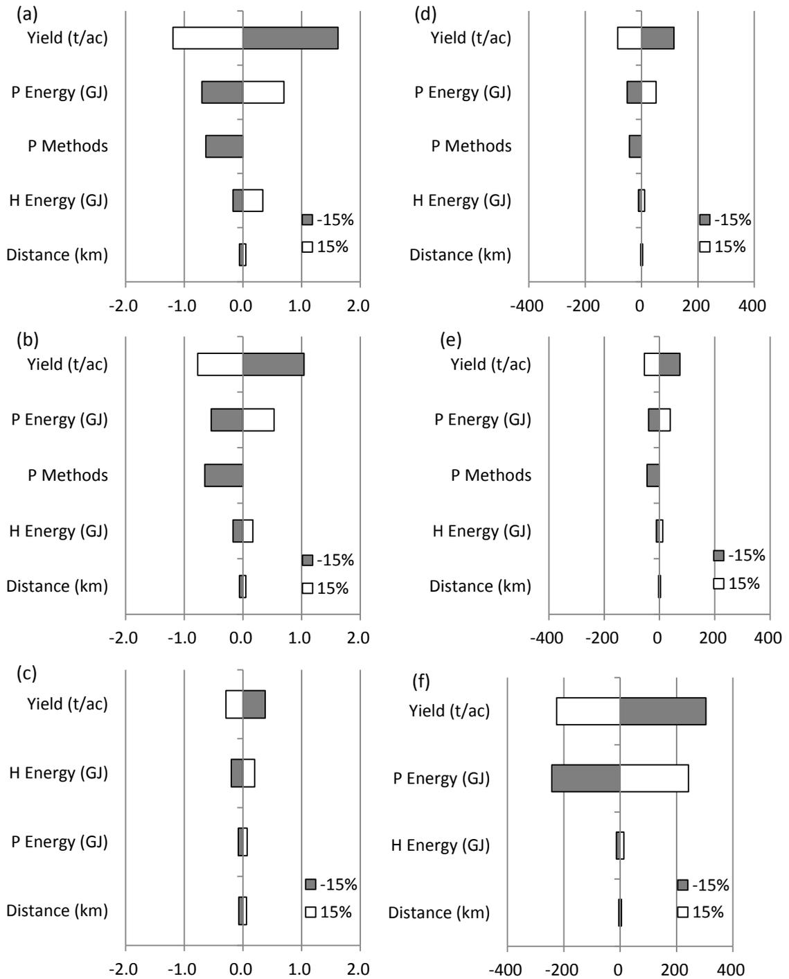
**Figure 5.5. (a), (b) and (c) fast pyrolysis, slow pyrolysis and Missouri kiln sensitivity analysis of total energy use (GJ/t); (d), (e) and (f) fast pyrolysis, slow pyrolysis and Missouri kiln sensitivity analysis of CO<sub>2</sub> equivalent emission (kg CO<sub>2</sub> eq/t)**
