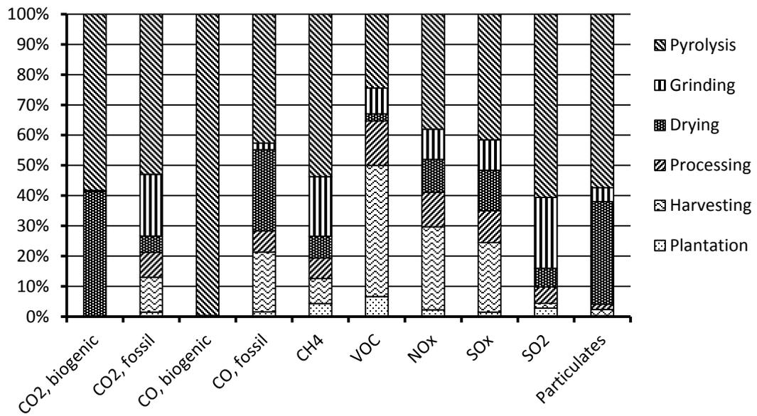
**Figure 5.4. Process contribution of fast pyrolysis to airborne emissions**
