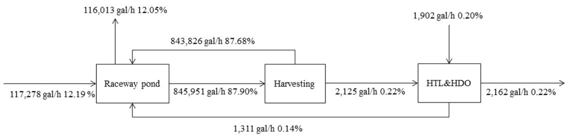
**Figure 3.2. Water balance of the open raceway pond for algae cultivation**
