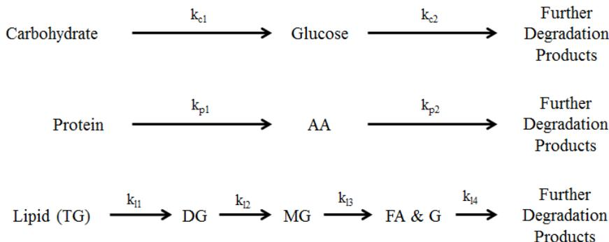
**Figure A.4. Schematic diagram of algae decomposition**
