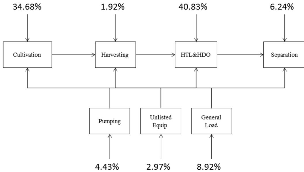
**Figure 3.3. Section contribution of the total electricity consumption of the algae liquefaction plant**
