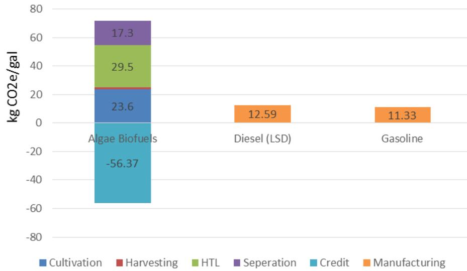
**Figure 4.3. Comparison of CO<sub>2</sub> equivalent emission of algae bio-crude, diesel and gasoline**
