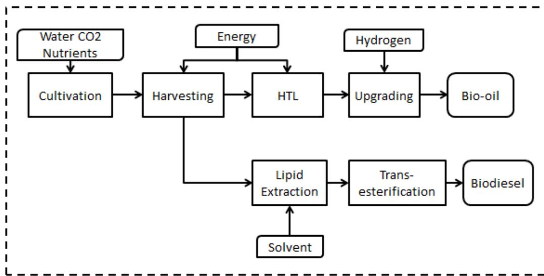
**Figure 2.7. System boundary of biofuels production from algae**
