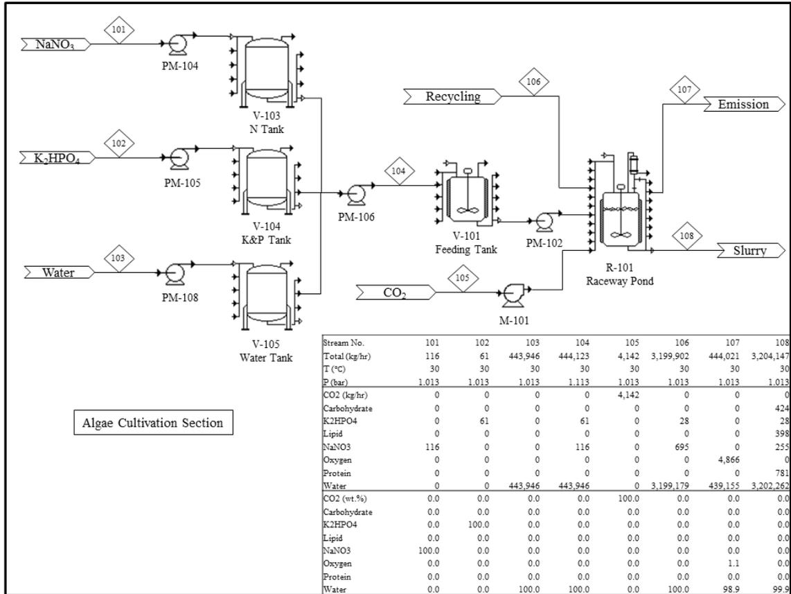
**Figure A.1. Process flow diagram and mass balance of algae cultivation**
