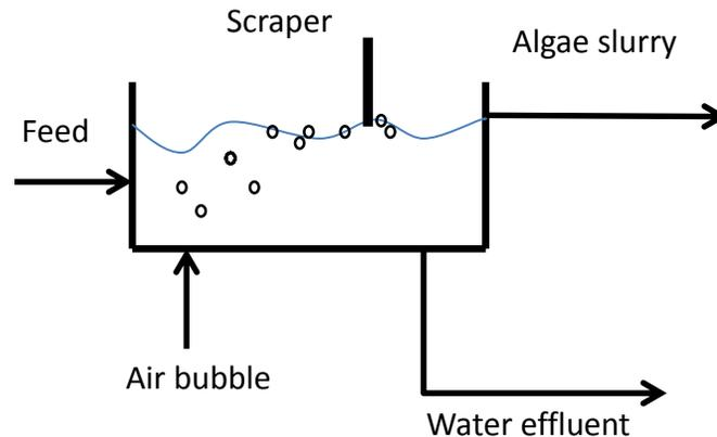
**Figure 2.3. Schematic diagram of dissolved air flotation**
