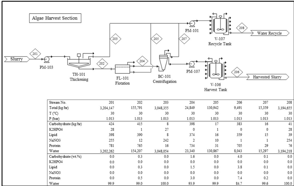
**Figure A.2. Process flow diagram and mass balance of algae harvest**
