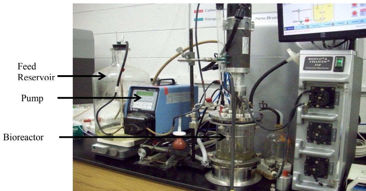
Figure 3.1: Set-up of continuous process (chemostat)
