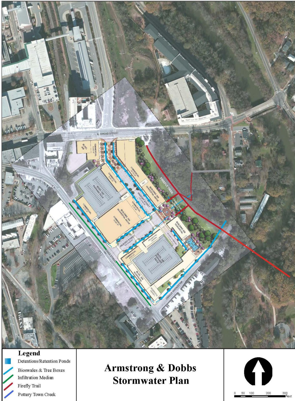
Figure 24: Stormwater Site Plan – Swales. The blue and green lines show possible locations for street side bioswales to transport and infiltrate stormwater. Dotted line segments denote pipes.
