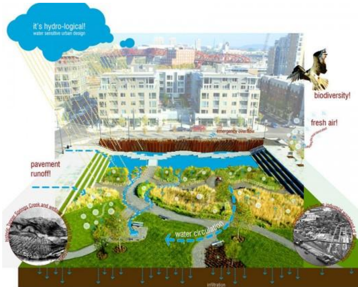
Figure 17: Water Circulation in Tanner Springs Park Image courtesy of Atelier Dreiseitl
