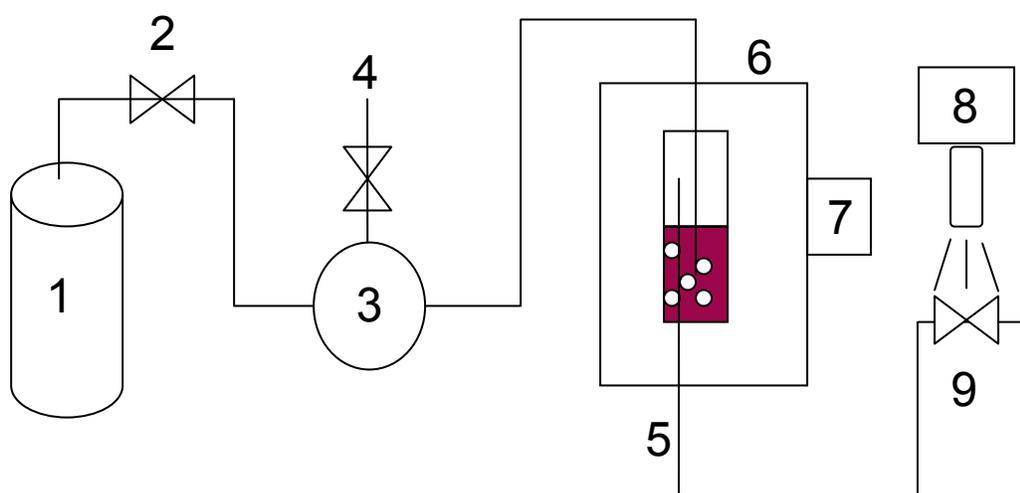
**Figure 3.1.** Supercritical carbon dioxide processing system. 1 is the dip tube carbon dioxide tank. 2 is the tank regulator. 3 is the high pressure pump (41.4MPa max). 4 is the air supply regulator. 5 is the venting carbon dioxide tube. 6 is the temperature controlled incubator. 7 is the PID controller. 8 is the heater. 9 is the venting valve.
