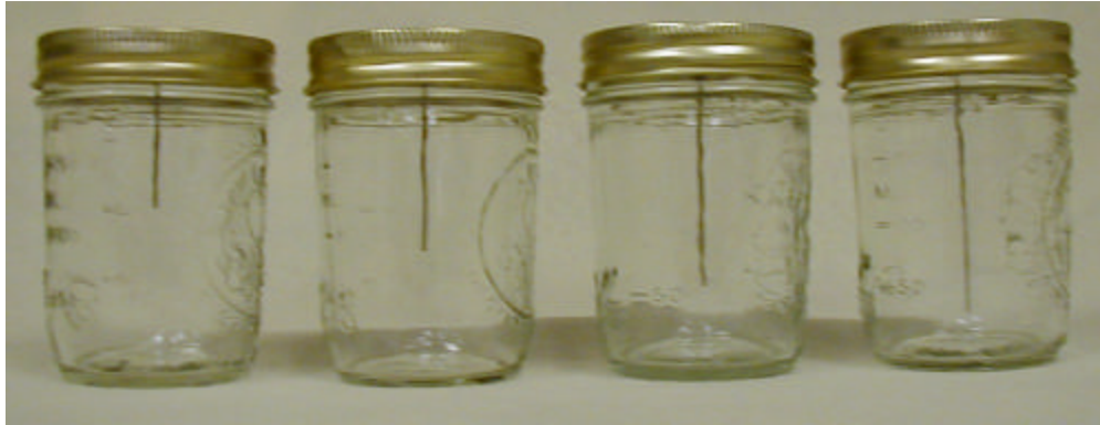
Figure 3.3. Four lengths of needle type thermocouples in half-pint jars
