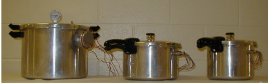
Figure 3.1. Retorts used in this study, from left to right: 17 qt, 8 qt, 6 qt
