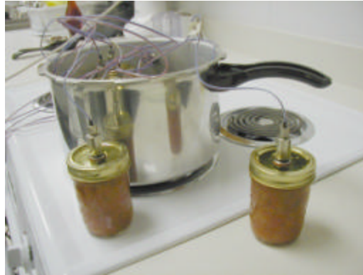
Figure 3.2. Internal leads attached to jar thermocouples
