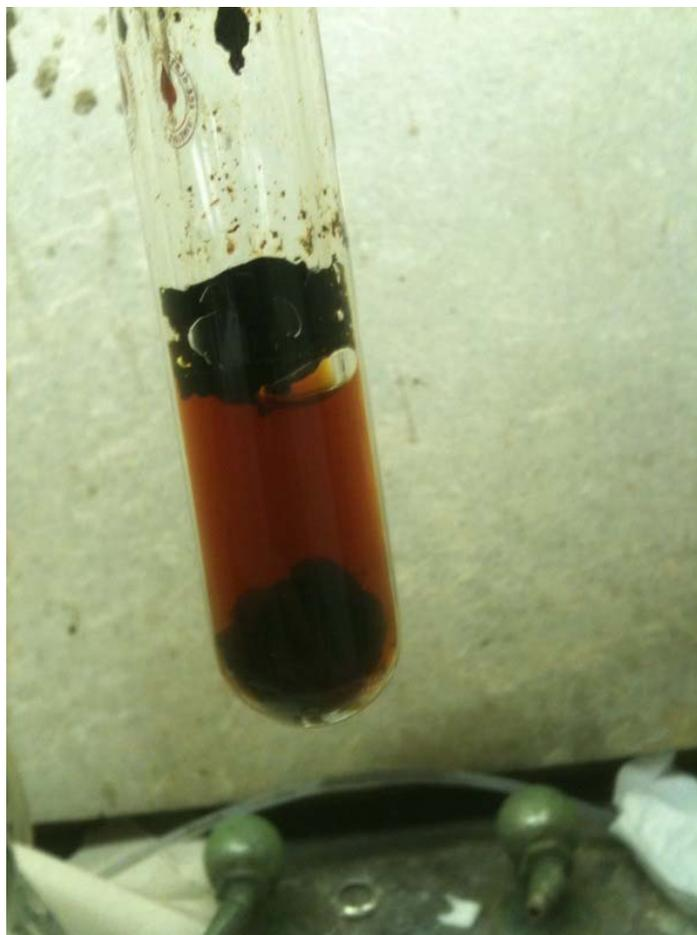
Figure 26. Solid disc formed over the hydrolysis products of ILC aqueous phase bio-oil and PCC catalyst.
