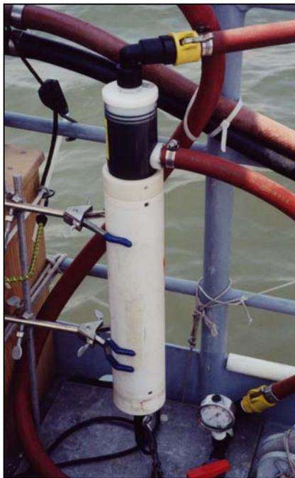
Figure 7. Multi-parameter sensor measuring the sediment-water interface.
