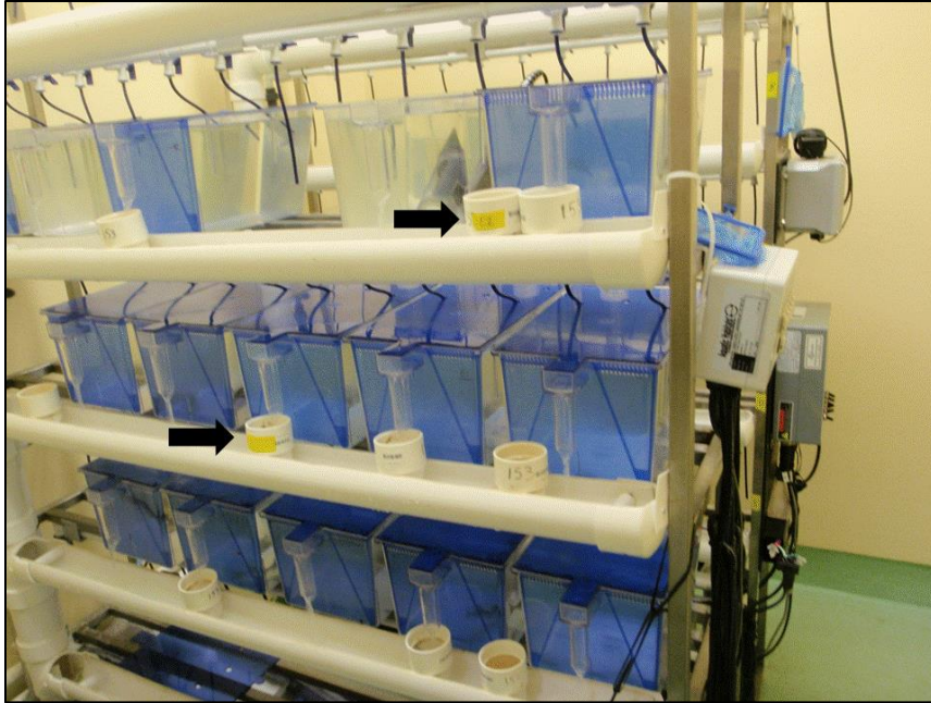
Figure 2.1. Recirculating aquaculture system (Aquatic Habitat, AHAB, Pentair Aquatic Eco-Systems) used to hold Atlantic sturgeon during mussel host trials. Note 153 \mu m mesh filter cups at tank outflows.
