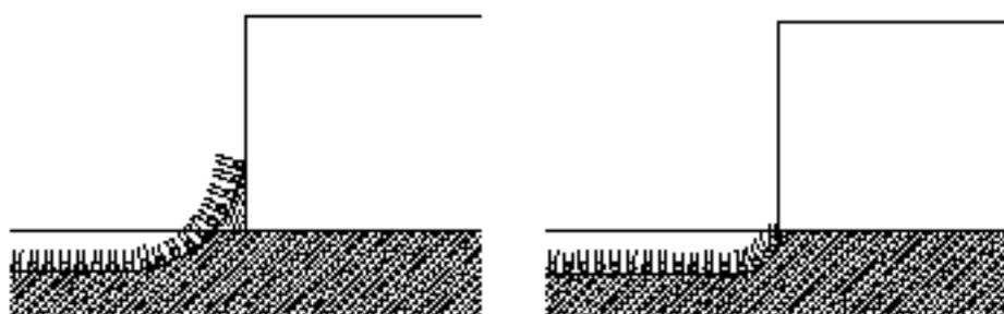
Hydrophilic Barrier (Delrin®)      Hydrophobic Barrier (Teflon®)
