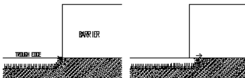
Hydrophilic Barrier (Delrin®)      Hydrophobic Barrier (Teflon®)
