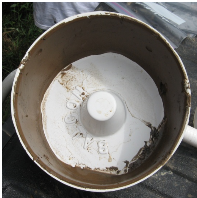
Centrifuge bowl with collected suspended sediment
