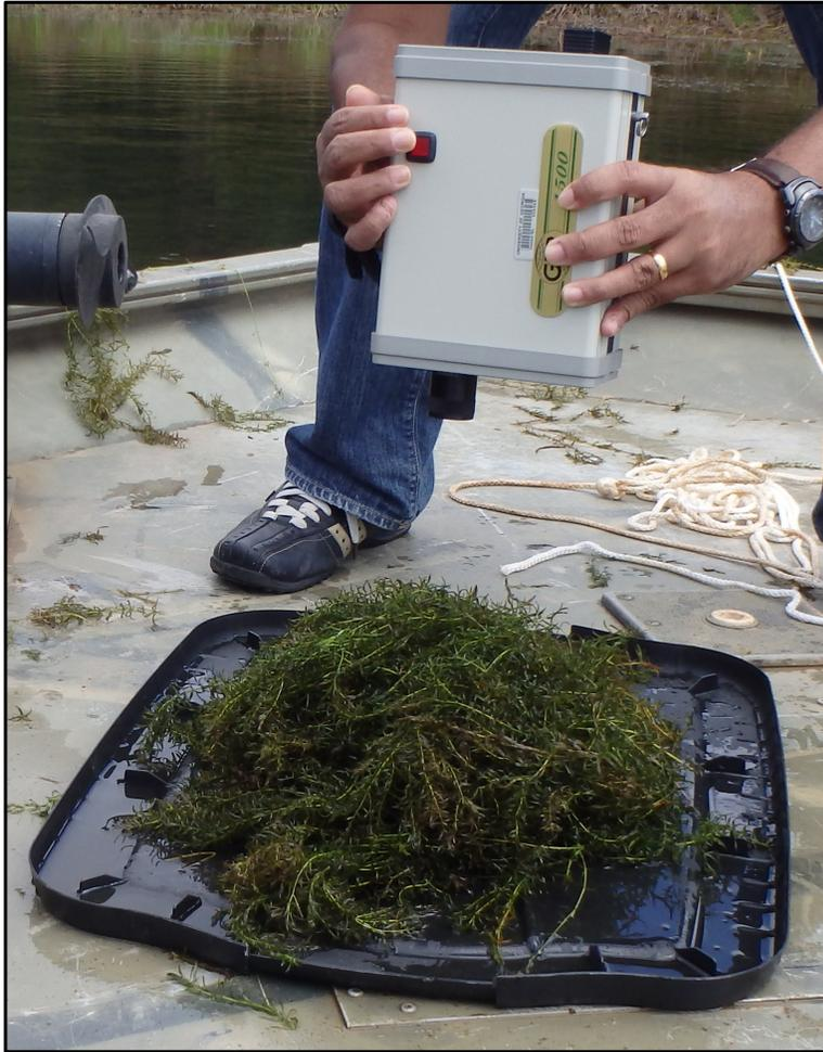
Figure 1.3: Collection of the reflectance values of harvested hydrilla with the Spectra Vista Corporation GER 1500.
