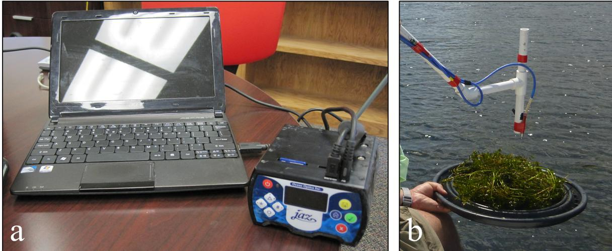
Figure 1.2: (a) Ocean Optics JAZ spectrophotometer connected to a field laptop. (b) Collection of the reflectance values of harvested hydrilla with the JAZ's submersible fiber optic sensor and frame.
