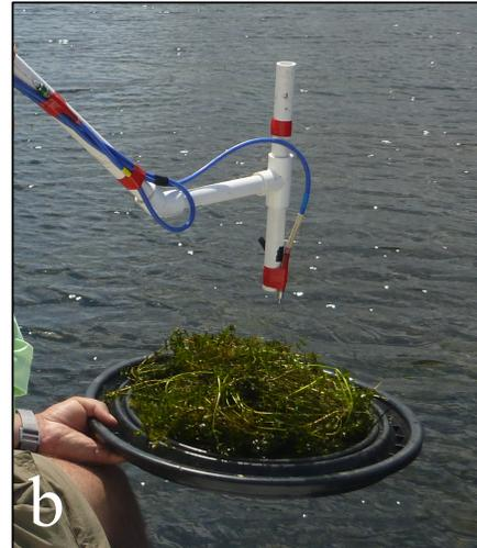
Figure 1.2: (a) Ocean Optics JAZ spectrophotometer connected to a field laptop. (b) Collection of the reflectance values of harvested hydrilla with the JAZ's submersible fiber optic sensor and frame.
