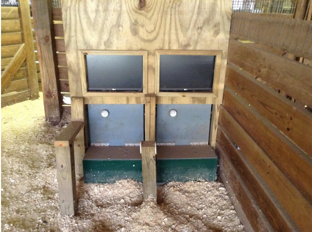
Figure 2.3. A photo of a retrofitted Deer-Training-Apparatus in a barn stall in the Whitehall Deer Research Facility, as seen by test subjects. The modifications include mounting LCD computer monitors in place of flashlights.
