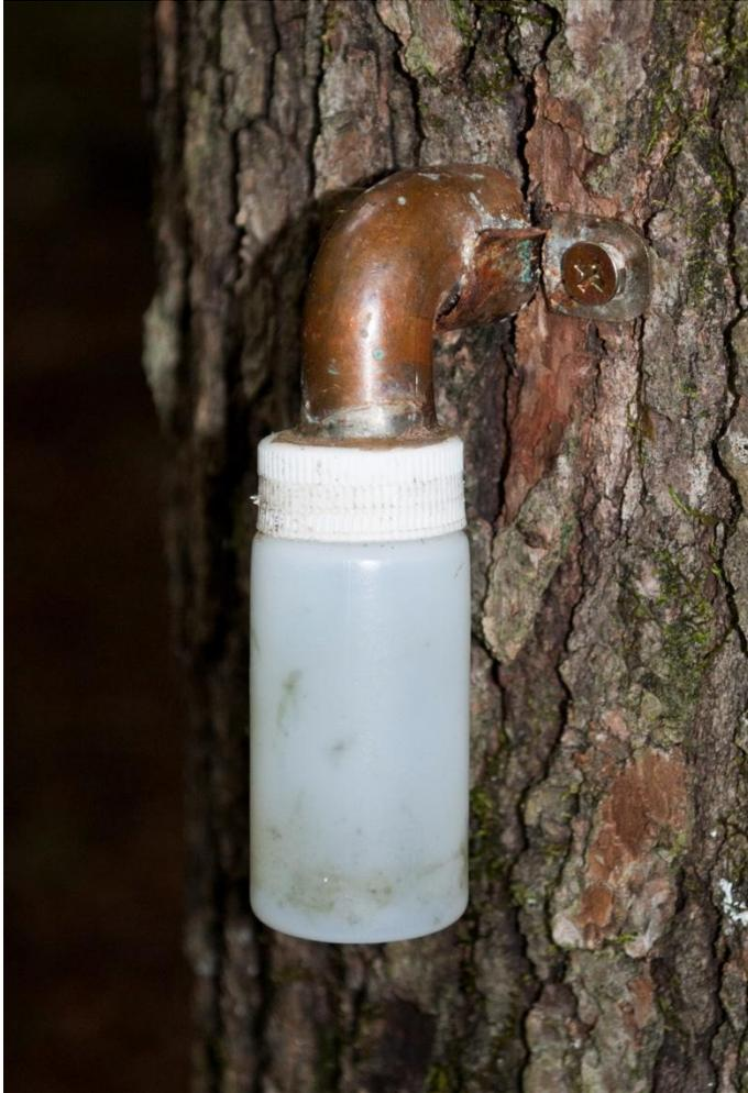
**Fig 2.1.** Emergence trap constructed from a 1.3cm diameter copper street elbow and pipe strap that was soldered to the elbow then the strap was cut part way through so the ends could be bent down to form attachment points to hold the trap to the tree.
