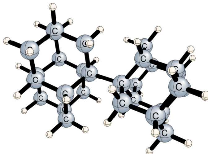
FIGURE 4.1: Optimized geometry of 1-(1-diamantyl) diamantane at the MP2/cc-pVDZ level of theory. The bridging C–C bond distance is 1.646 Å.
