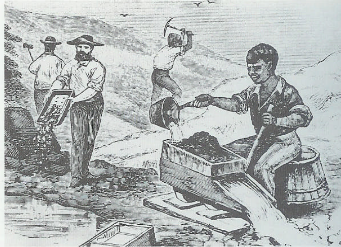
The cradle rocker was one of the most widely used placer mining devices in the Southern gold fields. Gold-bearing dirt was washed through a perforated plate, or "hopper," and riffle bars trapped small particles of gold in the lower trough. University of North Carolina Library.
