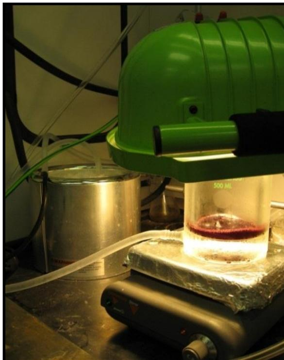
**Figure 3.03:** Set up for photo-oxidation reaction.
