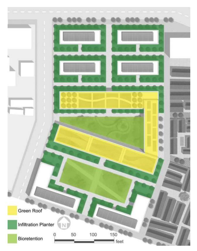
Figure 90. The location of three stormwater management systems
