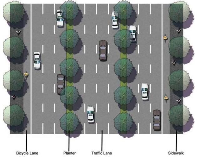
Figure 58. Level 1 road plan
