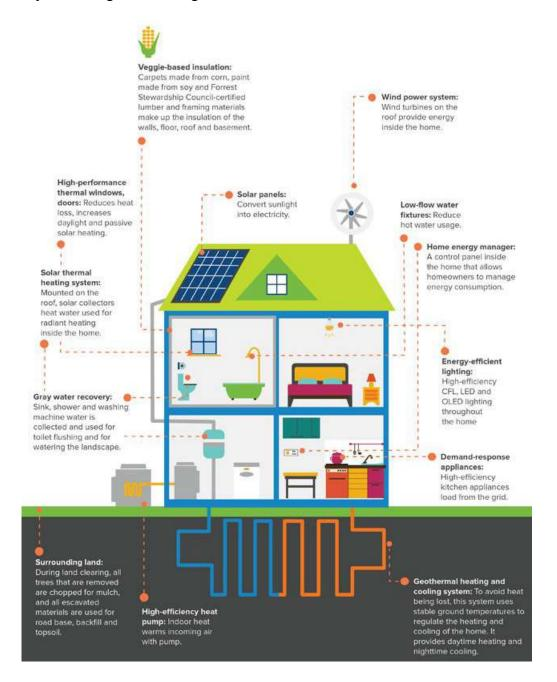
Figure 96. The operation system of a green building (Inhabitat n.d.)
