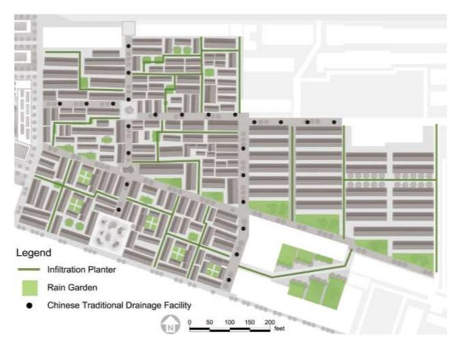
Figure 84. The distribution of drainage facilities
