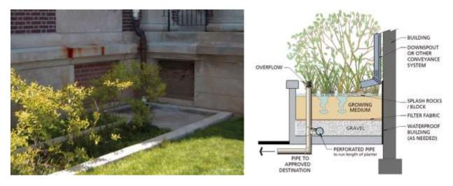
Figure 92. The infiltration planter (Meliora Design n.d.) and its structure (City of Portland n.d.)
