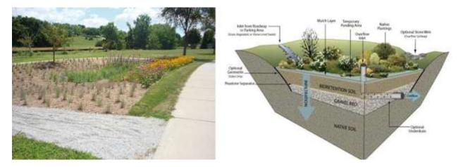
Figure 93. The bioretention (Omaha By Design n.d.) and its structure (Douglas County's Environmental Information Center n.d.)
