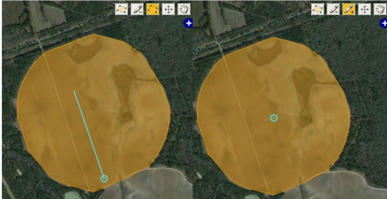
Figure 3.4: Illustrating adding a line (left) and a point (right) so that the created zones conform to field type and technology.
