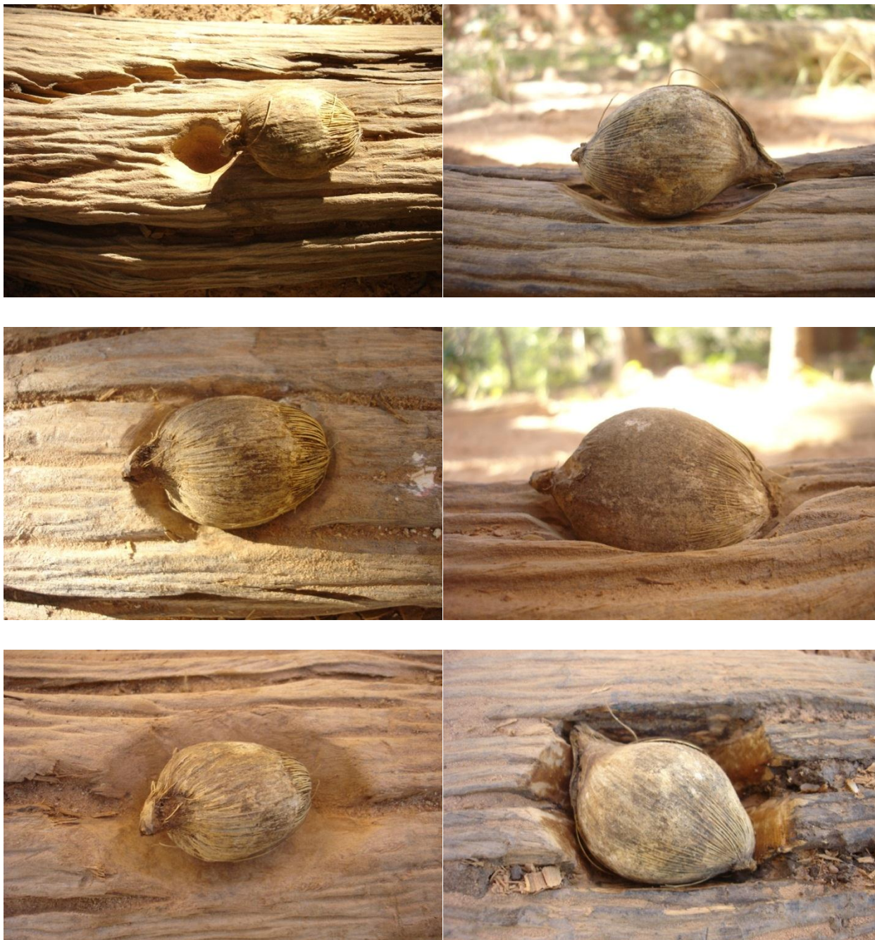
Figure 2.2. Photos of pits (left side from top to bottom: small, medium and large pit; right side from top to bottom: shallow, medium and deep pit)
