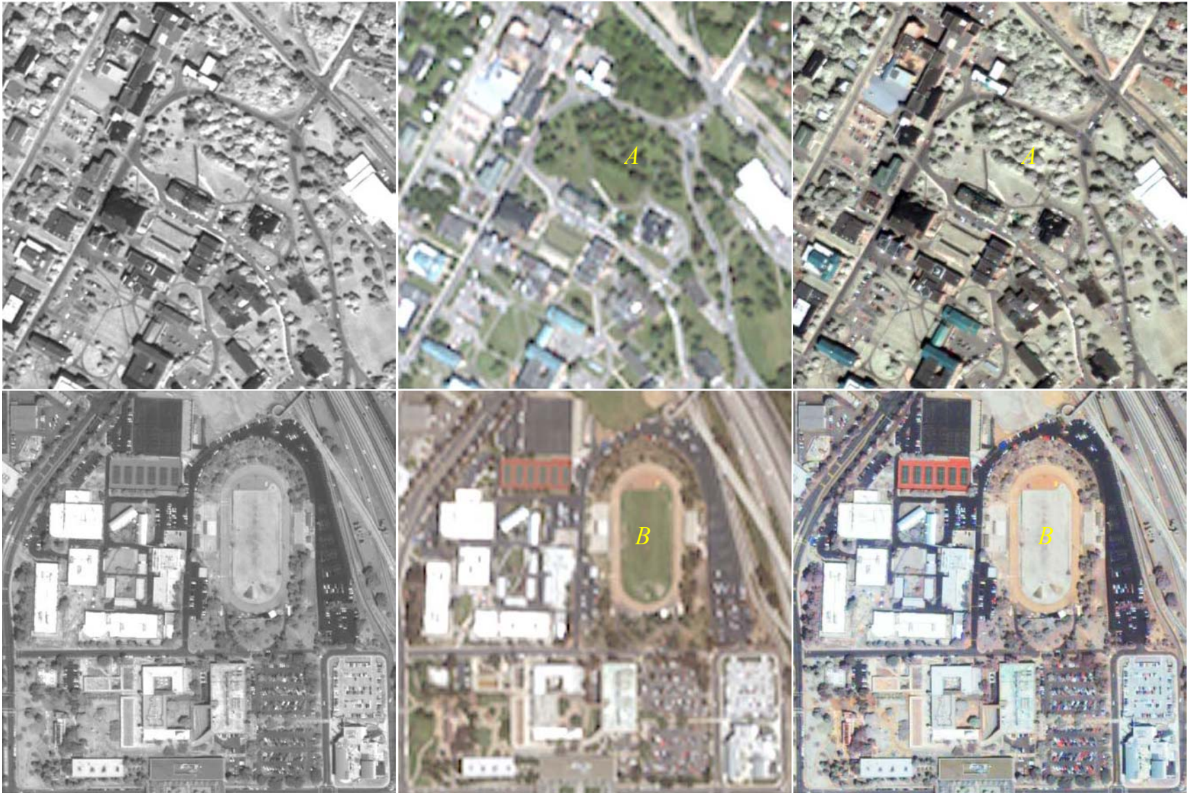
Figure 2.7: Different color distortions of the same IHS fusion algorithm and parameters. From left to right: original Ikonos Pan image with 1-m resolution, original Ikonos natural color images with 4-m resolution, and IHS fusion results. Top: Fredericton, Canada. Bottom: San Diego, the USA (Zhang 2002a).
