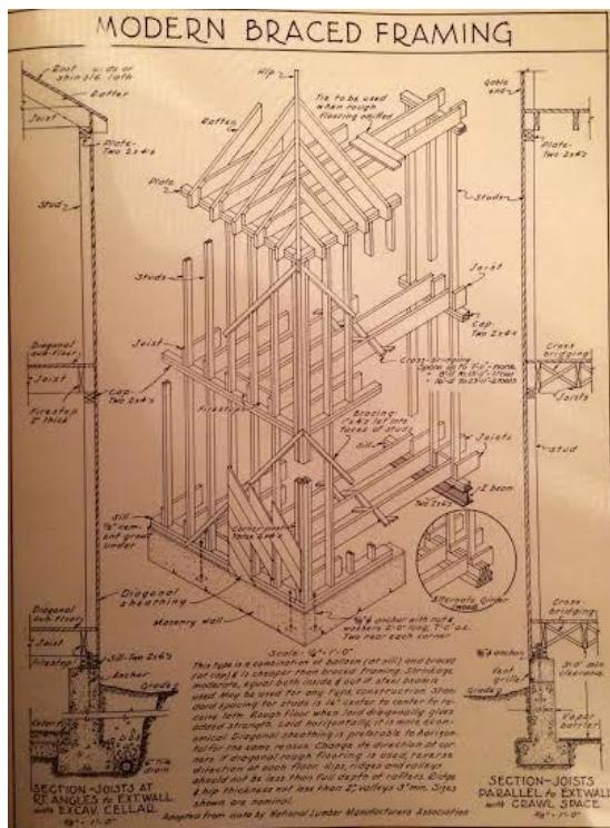
**Figure 21:** Modern Braced Framing
