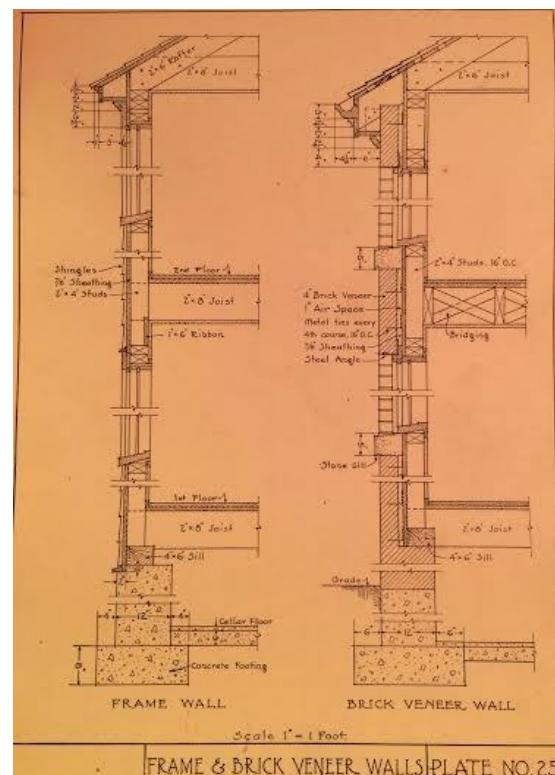
**Figure 14:** Frame and Brick Veneer Walls (Rouillion, 57)
