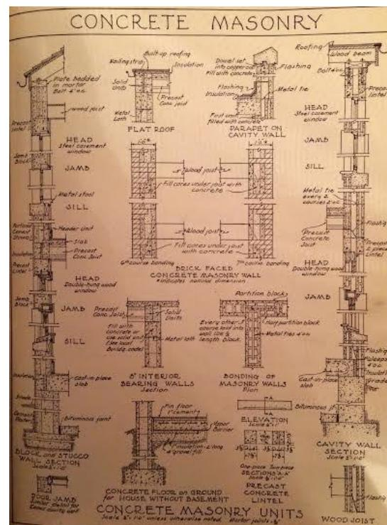
**Figure 24:** Concrete Masonry (1951 Ramsey, 37)
