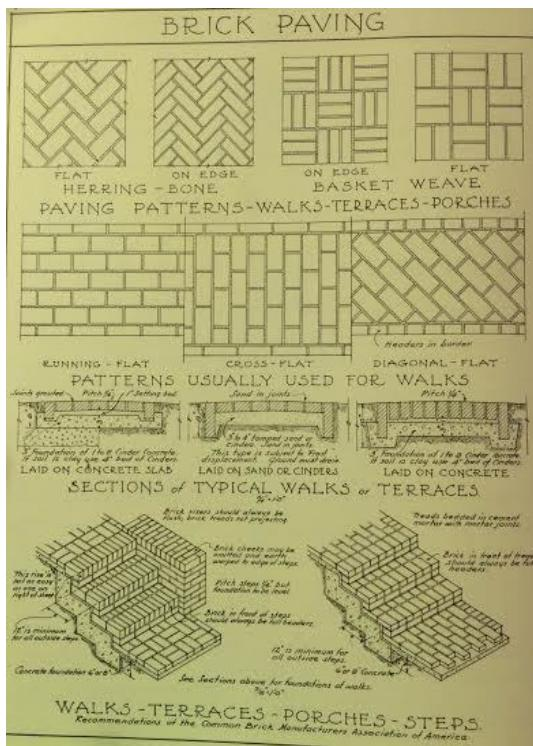
**Figure 8:** Masonry Flooring & Paving (1932 Ramsey, 5)
