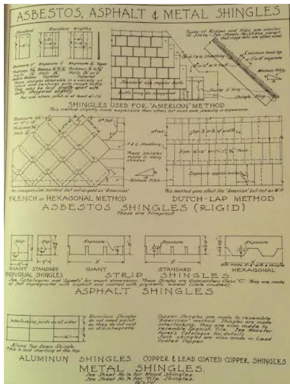
Figure 18: Asbestos, Asphalt, & Metal Shingles (1932 Ramsey, 77)
