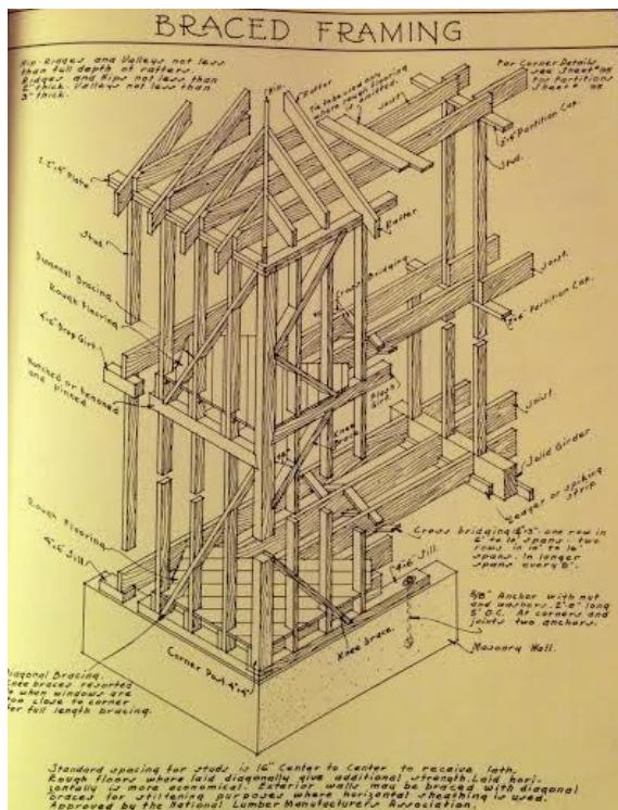
**Figure 11:** Braced Framing (1932)
