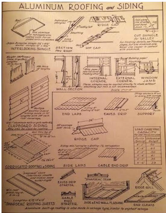
**Figure 28:** Aluminum Roofing and Siding (1951 Ramsey, 115)
