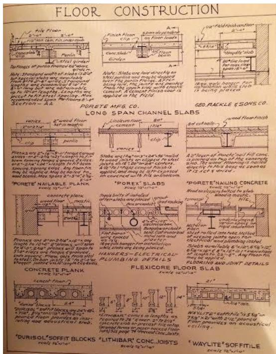
**Figure 27:** Floor Construction (1951 Ramsey, 79)
