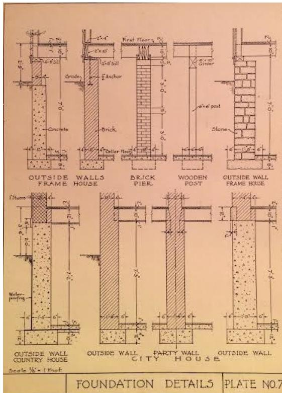
**Figure 10:** Foundation Details (Rouillion, 21)
