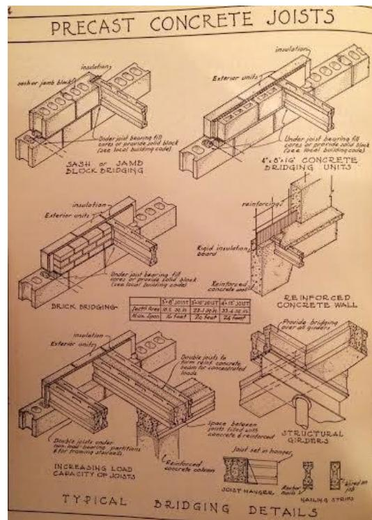
**Figure 26:** Precast Concrete Joists (1951 Ramsey, 74)
