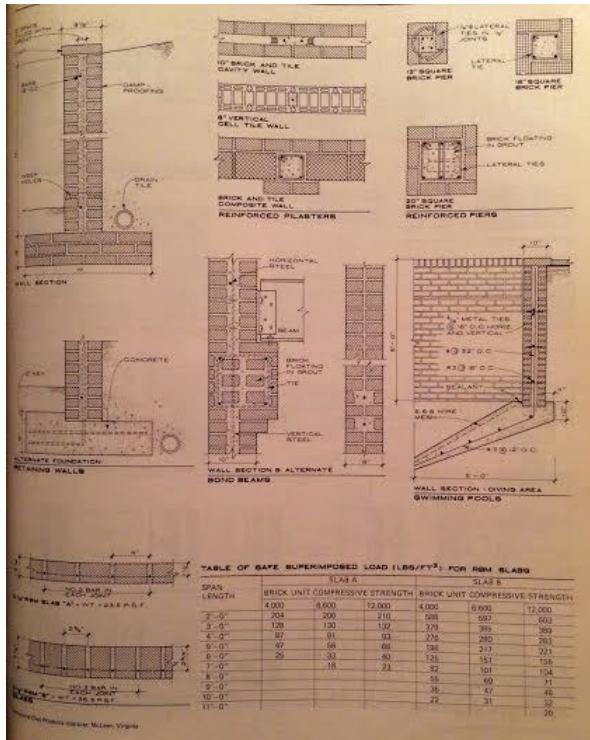
Figure 35: Reinforced Brick Masonry (1970 American, 155)
