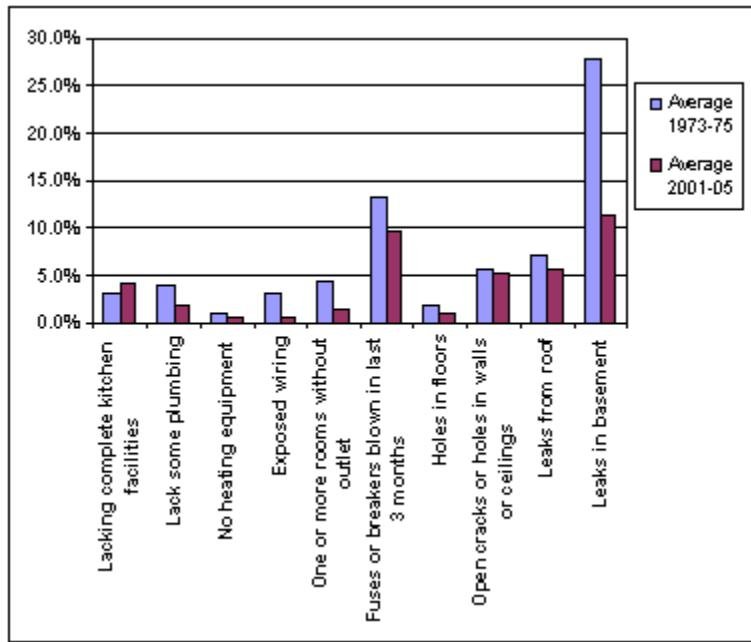
**Figure 7:** Selected Housing Defects from 1973-1975 and 2001-2005 and Rates of Occurrence at the Beginning and End of Each Period, from "32 Years of Housing Data" (Eggers, p. 18)
