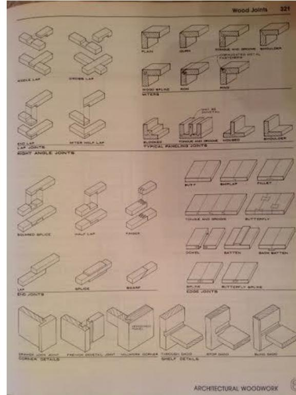
**Figure 47:** Wood Joints Figure 2 (1988 American, 321)
