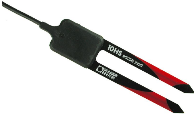
Figure 1-12. Decagon Device 10HS soil moisture sensor. A total of thirty-two sensors were used in the experiment.
