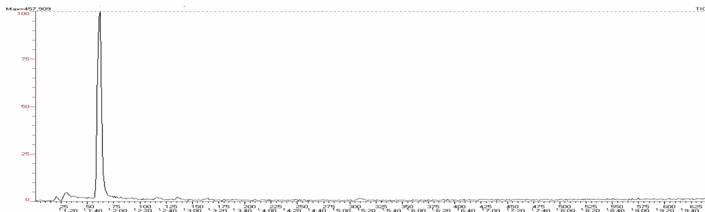
Figure 5.7. Headspace analysis (performed in triplicate) via GC/MS of the liquid phase of a wood fly ash/3-MB/O 2 only slurry (after 225 hours), Top ; a wood fly ash/3-MB slurry reacting in the presence of ClO 2 and O 2 (after 200 hours).
