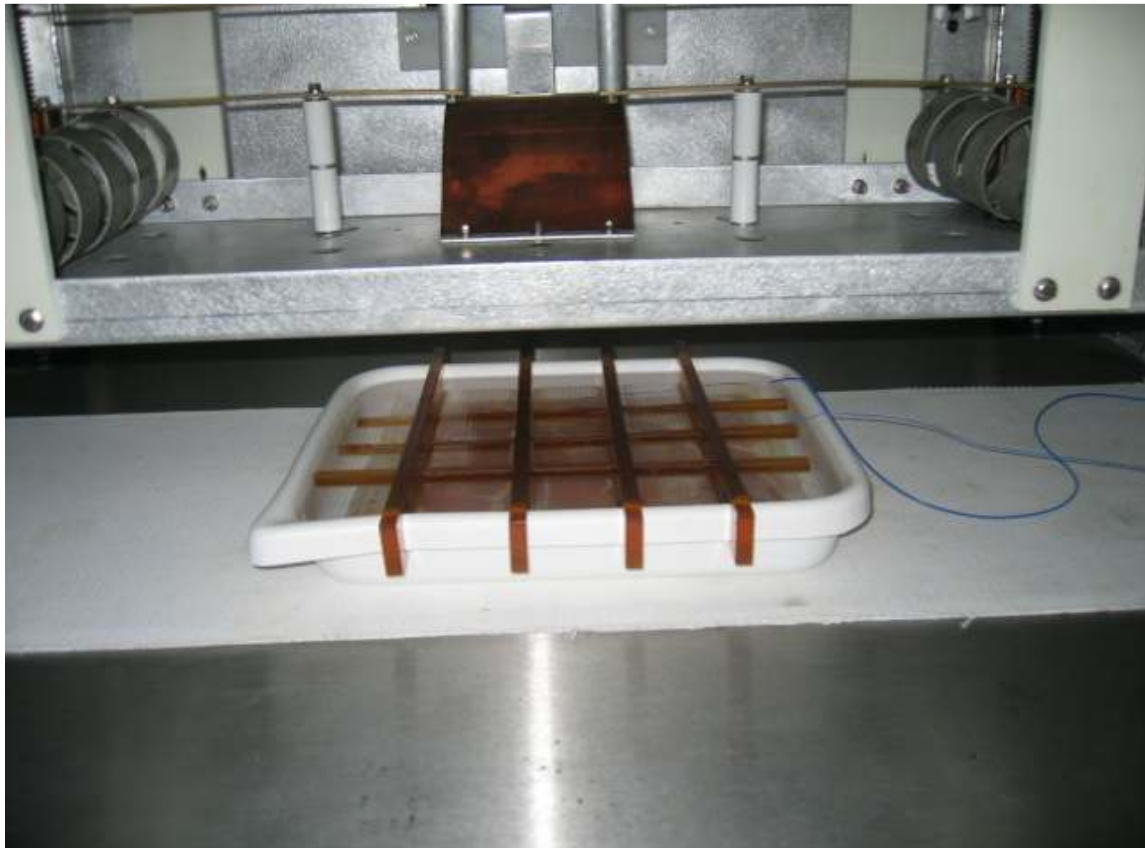
Figure 3.1 Container with grid in the RF oven
