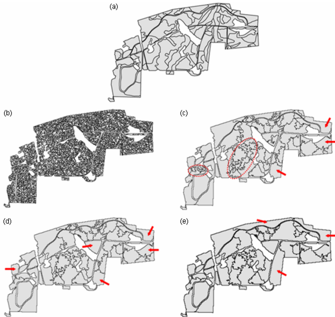
Figure 3.3. Over- and under-segmentation compared to manual interpretation: (a) manually-interpreted map, (b) over-segmentation at the scale of 4, (c) optimal segmentation at the scale of 18, and (d) optimal segmentation at the scale of 19, and (e) under-segmentation at the scale of 25.
