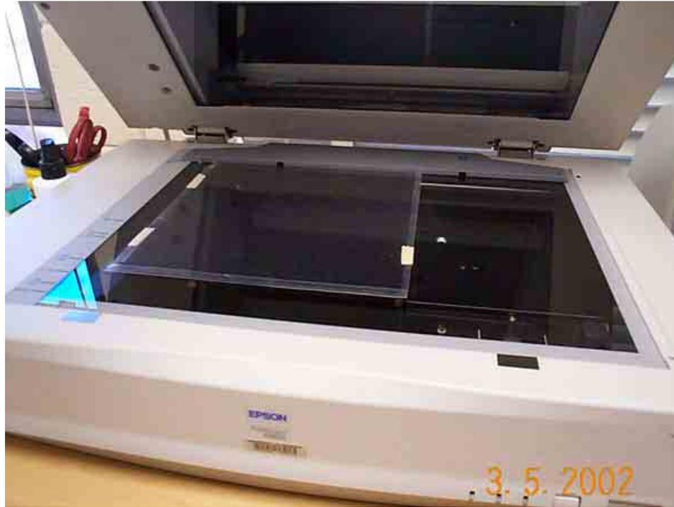
Figure 3-8. The photograph is placed on the bed of the scanner in preparation for scanning. A back-lighted transparency unit is required for scanning aerial photographs and overlays in film format.
