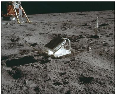
Figure 7.6. The Laser Ranging Retroreflector at Tranquility Base is a functioning scientific experiment (http://www.lpi.usra.edu/resources/apollo/images/print/AS11/40/5952.jpg)
