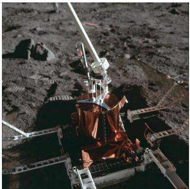
Figure 1.4. Seismic experiment equipment remaining at Tranquility Base (http://www.lpi.usra.edu/resources/apollo/images/print/AS11/40/5953.jpg)
