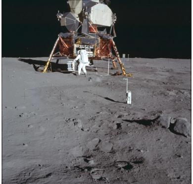
Figure 1.5. Apollo 11 Lunar Module, the bottom portion (descent stage) remains at Tranquility Base
