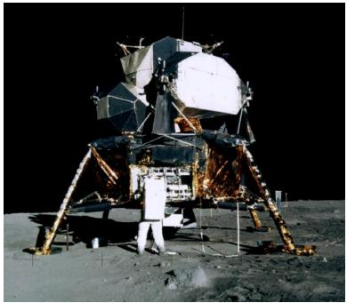
Figure 7.10. Apollo 11 Lunar Module, ascent and descent stages, the lower descent stage remains at Tranquility Base
