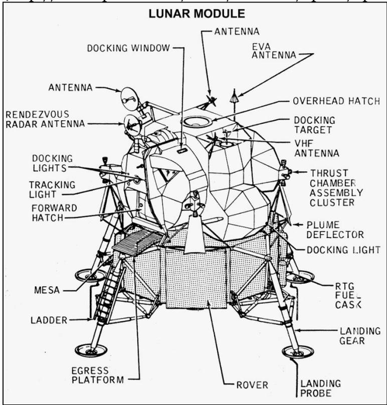
Figure 7.11. Lunar Module diagram, with shaded pattern identifying the descent stage that remains on the Moon
