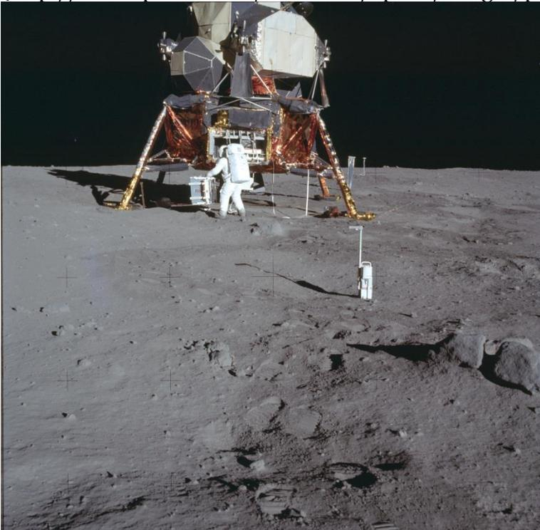
Figure 1.5. Apollo 11 Lunar Module, the bottom portion (descent stage) remains at Tranquility Base
